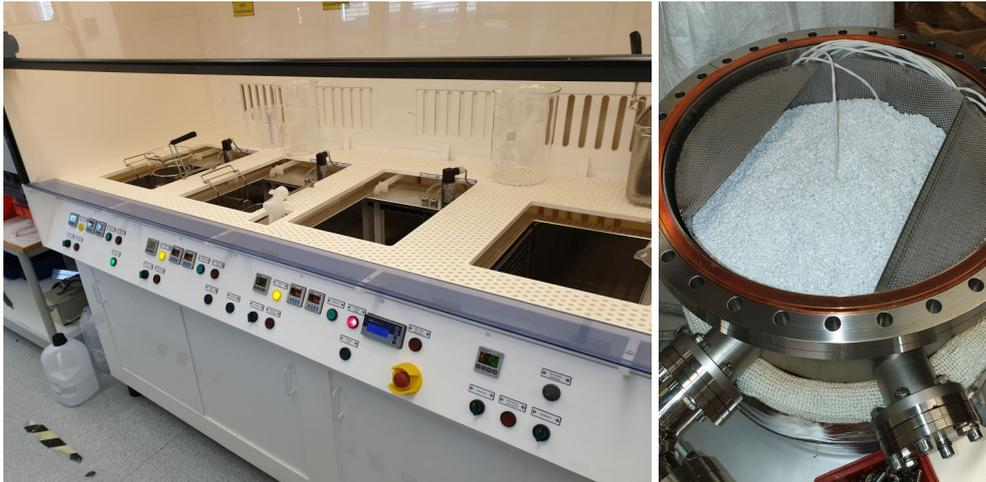
FIGURE 7.1: **Left:** Clean bench used for the PEN granulate cleaning. The three basins on the left were used for ultrasound cleaning while the one on the right was used for the cleaned granulate to dry. **Right:** Vacuum tank filled with cleaned and wet PEN granulate in a custom-made stainless-steel sieve. The white cables are used to connect temperature sensors.
