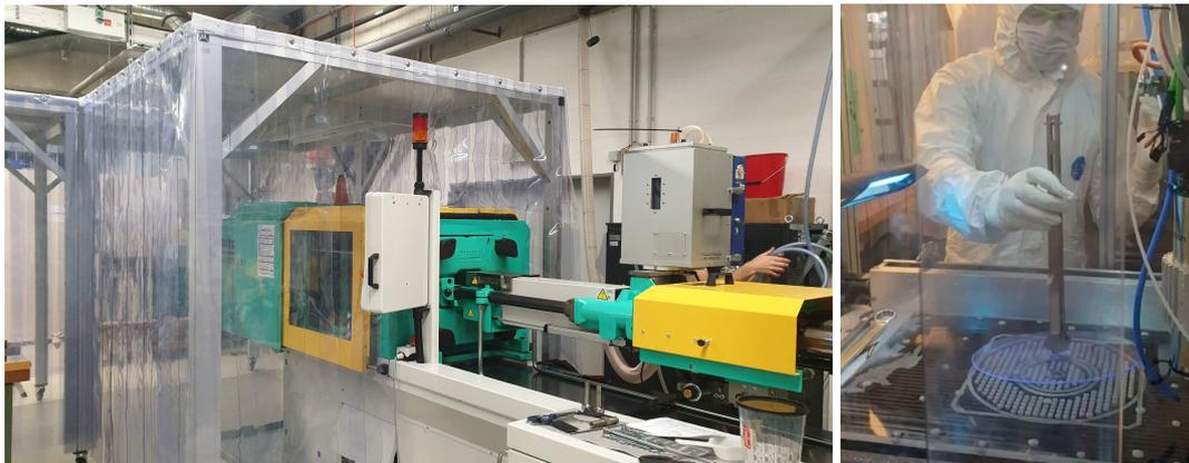
FIGURE 7.2: **Left:** Injection compression moulding machine used for the LEGEND-200 PEN production series. The class-1000 clean room tent contained all open parts of the machine. **Right:** CNC milling setup in the clean room tent. Picture taken while finished PEN disc was removed.
