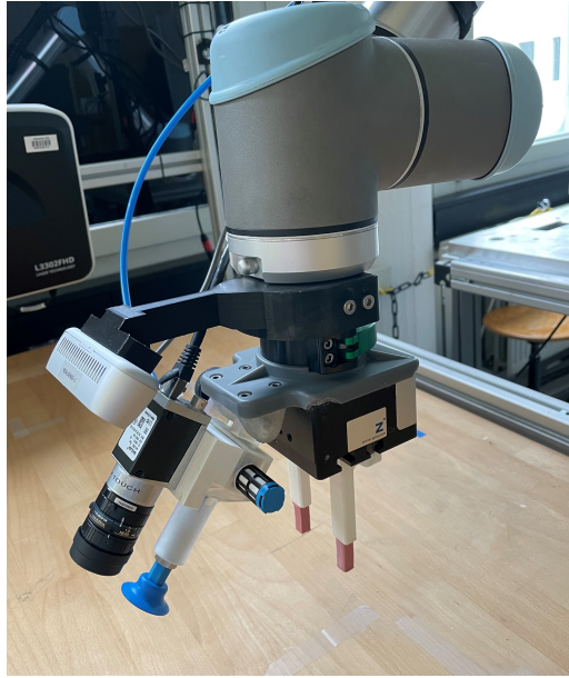
Figure 3.1: Eye-in-Hand Camera Setup. Cameras are mounted on the robot end effector, and move along with the robot motion.
