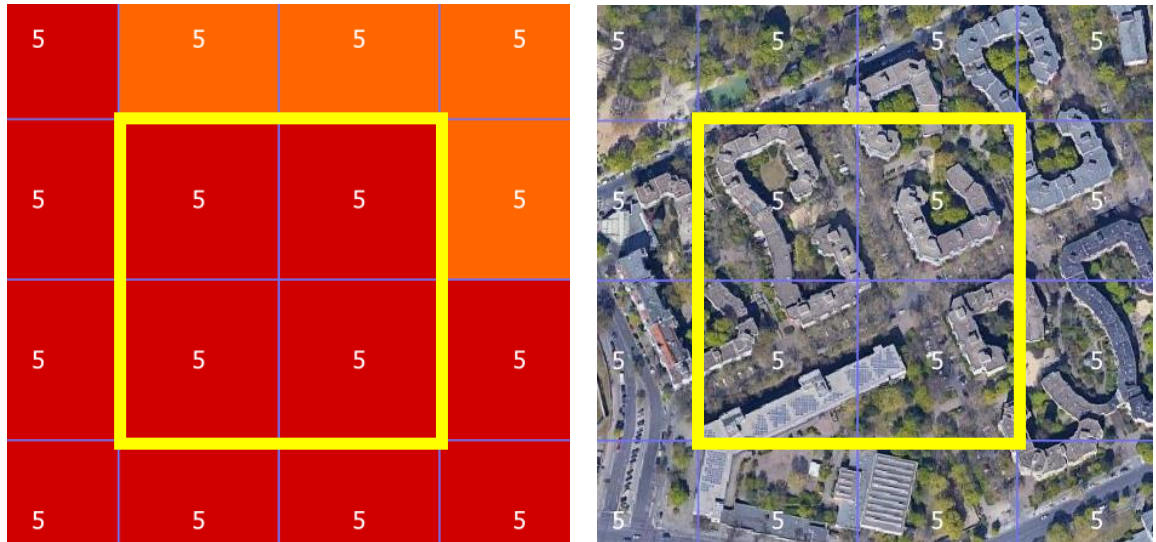
Figure 43. LCZ 2 in WUDAPT L0 and LCZ 5 in GIS-LCZ. Left image: color represents WUDAPT L0 and label represent GIS-LCZ. Right image: satellite imagery from tiles of the left image. (id: 76418 in shapefile)
