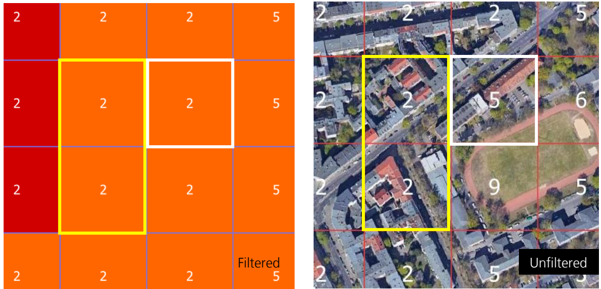
Figure 44. LCZ 5 in WUDAPT L0 and LCZ 2 in GIS-LCZ. Left image: color represents WUDAPT L0 and label represent GIS-LCZ. Right image: satellite imagery from tiles of the left image with the unfiltered GIS-LCZ as label. (id: 74444 in shapefile)
