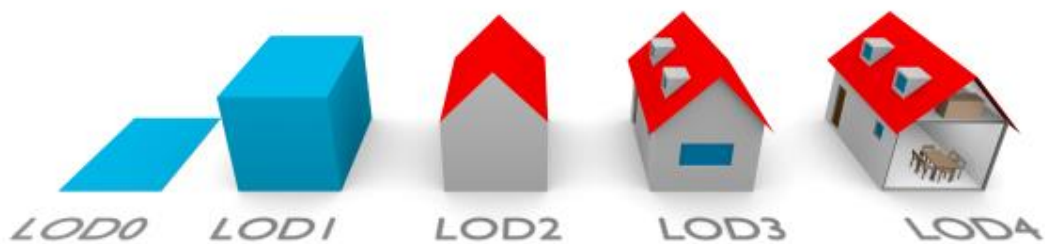
Figure 10. The five LODs of CityGML version 2.0 (Biljecki et al. 2016)
