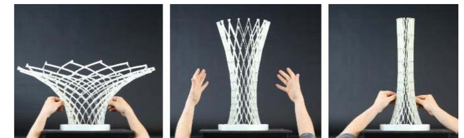
Fig. 19: Sequence of the umbrella opening and closing
