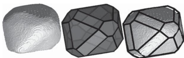
**Figure 8.** Left: micro-computed tomography image of crystal 1 after 17 min of growth; center: geometric crystal model (Figure 2) fitted to the crystal; right: combination of crystal image and fitted model.
