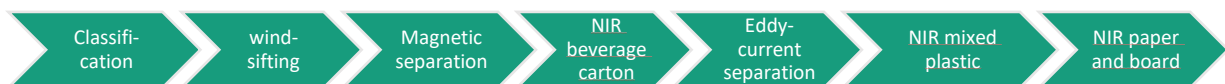
Figure 3. Overview of the individual process steps involved in sorting post-consumer plastic packaging. Adapted from [20]
