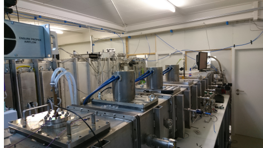
Figure 25: Picture of the used sputter facility. The clean room tent with the loading section of the facility is located behind the door.
