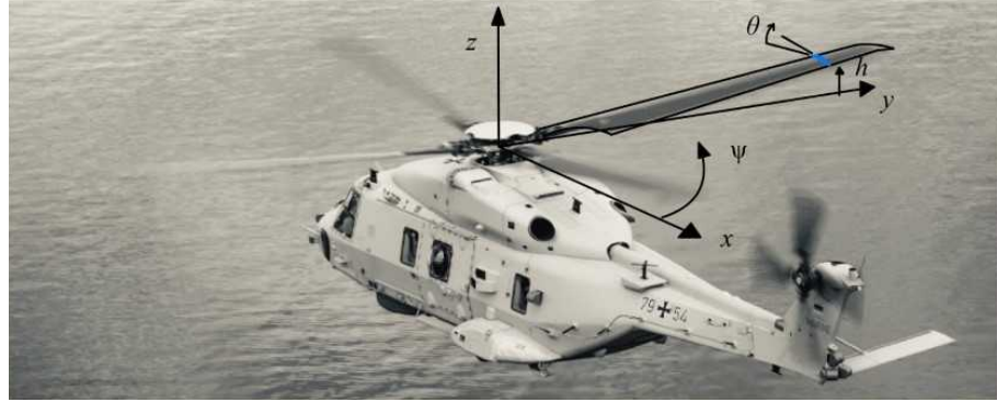
Figure 1.1: Illustration of the movement of a blade section (highlighted in blue) on a forward-flying NH-90 Sea Lion helicopter. [13]
