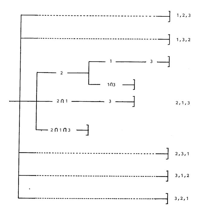
Figure 2: Failure tree of a 3-components system
