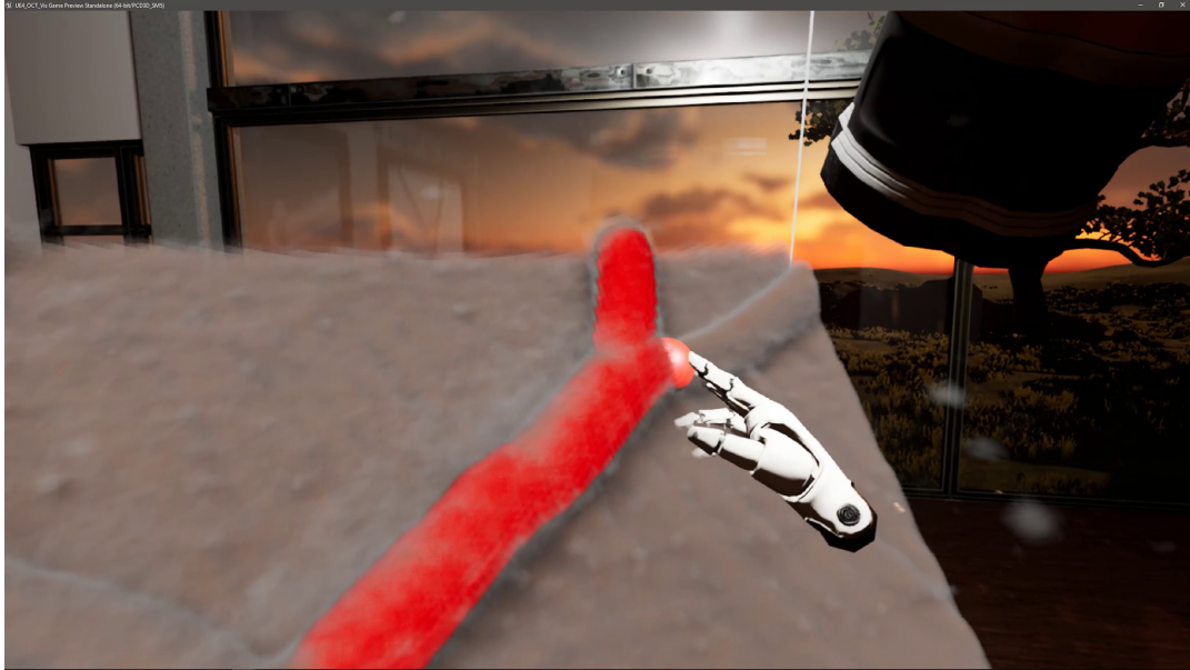
Fig. 5.5. Screenshot of the VR Planning application, showing intuitive volume annotation of risk areas using the tracked HTC Vive controllers, represented as hands in the virtual space.
