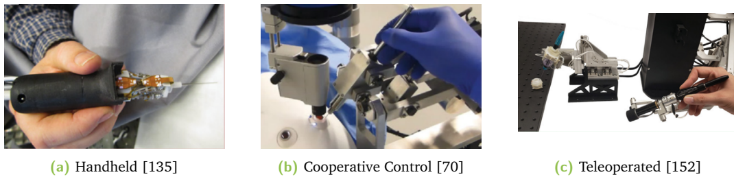
Fig. 2.7. Examples for the three major classes of microsurgical robots: the handheld Micron robot from Carnegie Mellon University (a), the cooperative control system developed at KU Leuven (b) and the teleoperated micromanipulator developed at the University of Utah (c).
