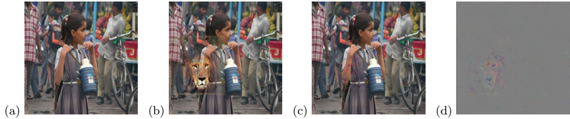
Figure 3.11: Placing salient patches. (a) Original image, label "water bottle". (b) Starting point containing a salient patch of the target class, classified as the target label "lion". (c) Final adversarial example after running a Biased Boundary Attack, also classified as "lion". (d) Difference image.
