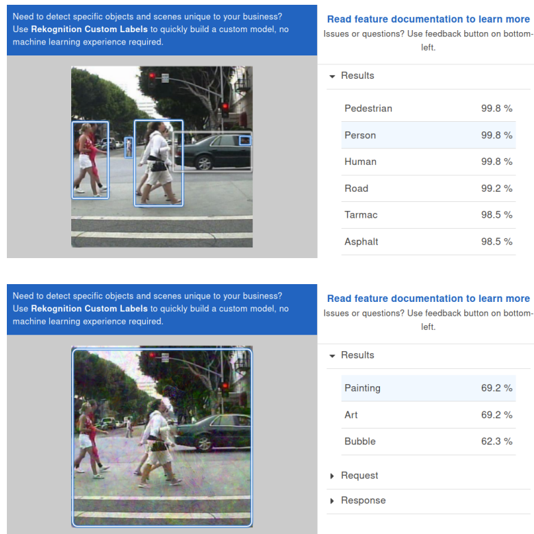
Figure 5.9: Making pedestrians disappear for Amazon Rekognition. (Top): Original image. The list of predictions contains "pedestrian", "person" and "human". (Bottom): Adversarial example, obtained after 3000 queries with the Biased Boundary Attack. All labels that hint at pedestrians are gone from the prediction list. Although the perturbation is visible to the human eye, it still causes the service to completely disregard the humans present in the picture.
