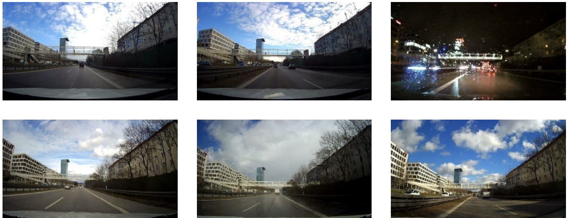
Figure 1.3: Natural perturbations on images of a driving scenario. All images have similar contents (same road) but differ significantly in environmental conditions (weather, day/night). Even though the images look extremely different on a per-pixel level, their semantics are very similar. An automated driving system would be expected to perform the same function, i.e. be robust to these changes. In some cases, there could be a difference – perhaps more careful behavior in darkness – but the system should be largely invariant to cloudy or sunny weather. As a result, such environmental changes are expected and fall under the category of natural perturbations. Taken from Cheng et al. [11].
