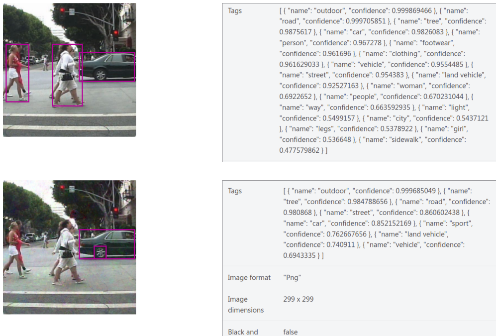
Figure 5.8: Making pedestrians disappear for Microsoft Azure. (Top): Original image. The list of predictions contains "person", "footwear", "clothing", "woman", "people", "legs", "girl". (Bottom): Adversarial example, obtained after 3000 queries with the Biased Boundary Attack. All labels that hint at pedestrians are gone from the prediction list.
