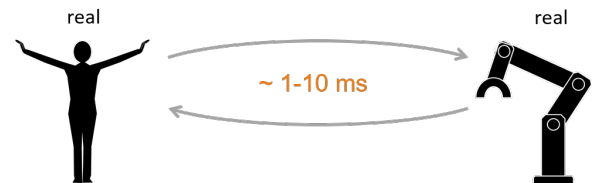
Fig. 2a: Direct remote control of a robot with strict ultra-reliable low-latency (URLLC) requirements
