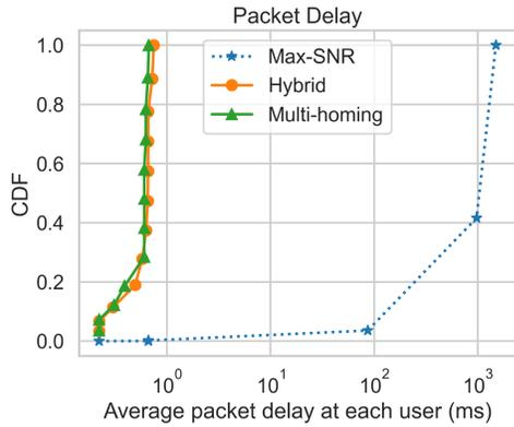
Fig. 8. CDF of average packet delay for a high traffic scenario
