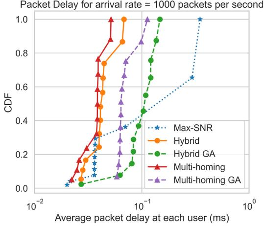
Fig. 4. CDF of the average packet delay for an arrival rate of 1000 packets per second
