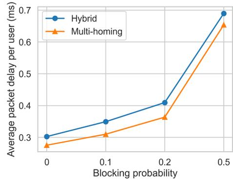
Fig. 6. Average packet delay for varying LiFi LOS blocking probabilities for a Hybrid and Multi-homing Network
