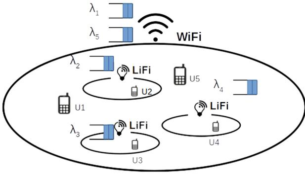
Fig. 1. Architecture of a LiFi-RF HetNet with QoS traffic
