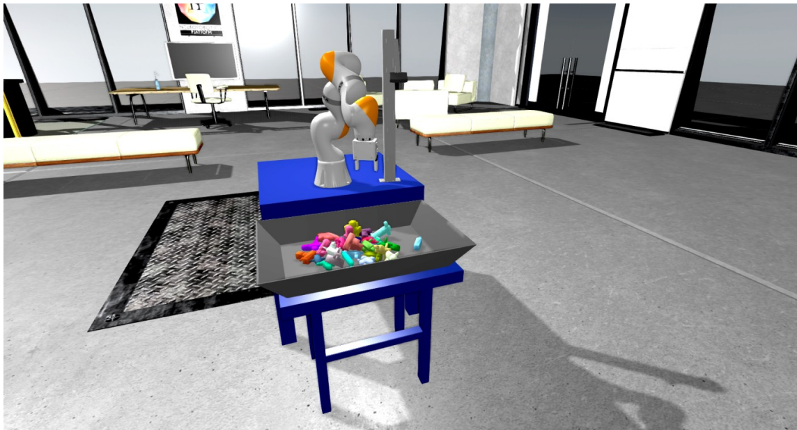
Figure 4.3: Digital twin of the robot grasping experiment in the NRP “Holodeck”, a digital lab space for virtual neurorobotics experiments. A KUKA LBR iiwa robot equipped with a Schunk PG 70 parallel gripper is placed next to a tray with random objects. The content of the tray is captured by an RGB camera mounted behind the robot.
