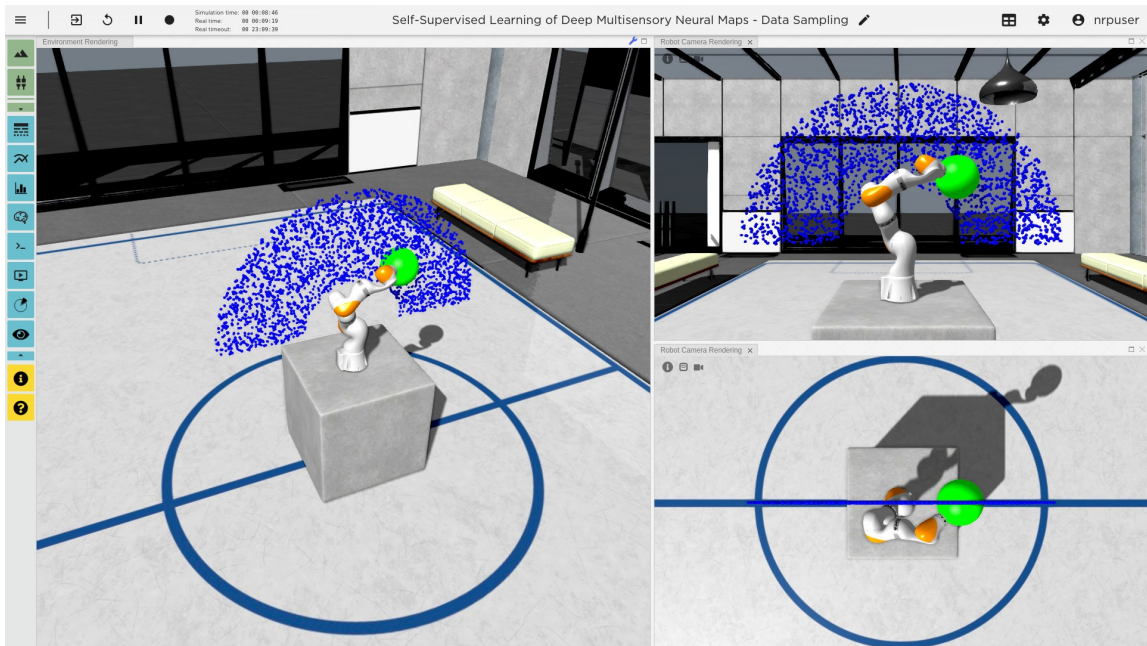
Figure 5.5: NRP experiment for the collection of multimodal training data as required by deep multisensory neural maps. The setup is based on the KUKA LBR iiwa robot model introduced in Section 4.1. Instead of a gripper, a green sphere is attached to the robot’s last link in order to provide a salient visual stimulus that indicates the workspace position. The blue dots are a visualization of the sampling space and correspond to samples from the multimodal data set D_{map} . The insets on the right display additional camera views of the scene. During data collection, joint angles ( proprioception ) and camera data ( vision ) are recorded simultaneously.
