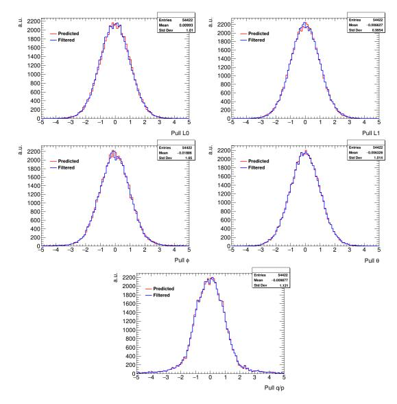
Figure 8.10: Pull distributions of predicted and filtered parameters at the corresponding measurement surfaces in the tracking detector with 10 GeV initial momentum. The statistics refer to the filtered distributions.
