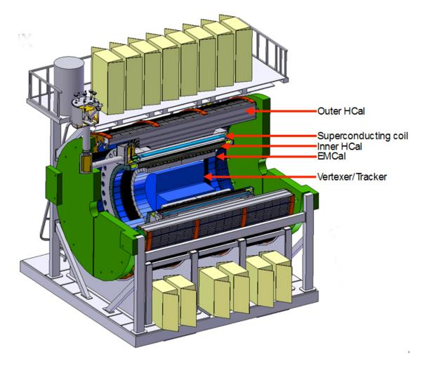
Figure 8.8: Schematic overview of the sPhenix detector. The interaction point lies in the centre of the detector. The figure is taken from Reference [138].
