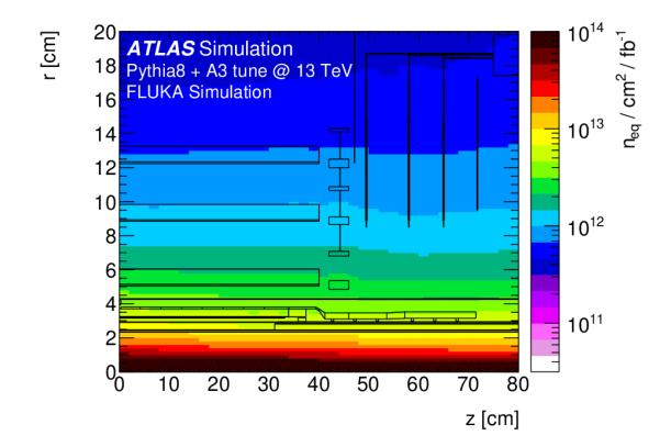
Figure 3.21: Simulated prediction of a 1 MeV neutron-equivalent flux per  $fb^{-1}$  in the silicon detectors of the ATLAS ID. The plot shows a one-quarter slice (z > 0 cm and above the beam) of the radial distance from the geometrical centre of the detector [81].
