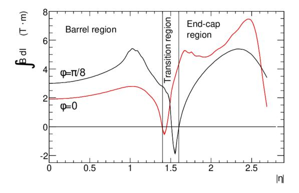
**Figure 3.20:** Bending power in the toroidal magnetic field versus  $|\eta|$  [59].
