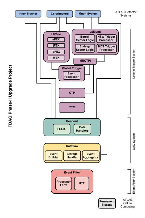
Figure 3.25: ATLAS Phase-II TDAQ design showing the sub-systems involved and their connection among each other as well as the connection to the detector systems. For simplicity the connection between components of a system are not drawn [89].
