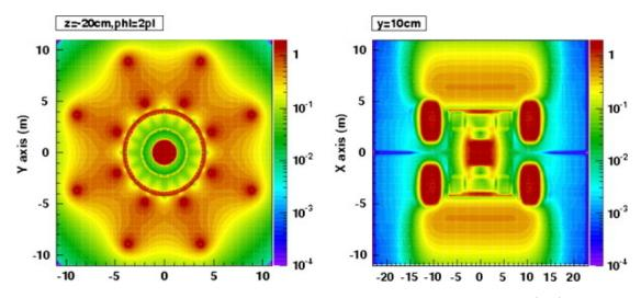
Figure 3.19: Magnetic field map of the ATLAS experiment in *x-y*-direction (left) and *z-x*-direction (right) [79].
