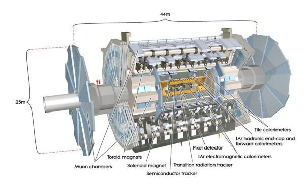
Figure 3.12: Cutaway overview of the ATLAS detector and the individual components [60].
