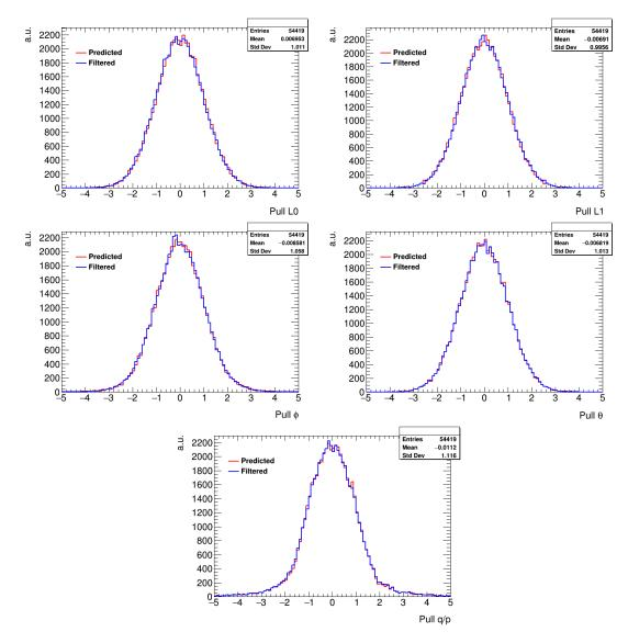
Figure D.17: Pull distributions of predicted and filtered parameters at the corresponding measurement surfaces in the tracking detector with 5 GeV initial momentum. The statistics refer to the filtered distributions.
