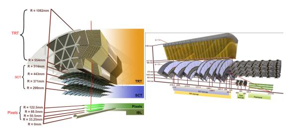
Figure 3.15: Schematic overview of the ID components in the barrel (left) and the end-caps (right) and their nominal distance to the centre of the beam-pipe [63, 64].
