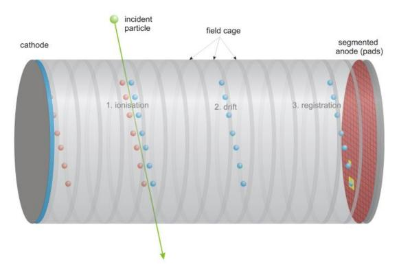
Figure 8.1: Schematic illustration of the TPC detection principle [131].
