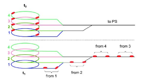
Figure 3.5: Beam extraction scheme from Proton Synchrotron Booster. The phases of individual bunches from the four rings are synchronised until the time  $t_0$ . Afterwards one ring after another is emptied starting with Ring 3, then 4, 2 and 1. This figure is taken from Reference [37]
