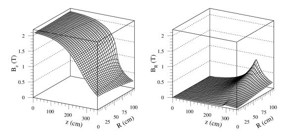
Figure 3.14: Solenoidal magnetic field strength in longitudinal direction (left) and radial direction (right) as a function of the position in the r-z-plane [62].
