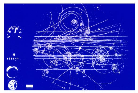
Figure 4.1: Photography of 16 GeV charged pions entering CERN's first liquid hydrogen bubble chamber in 1960 [94].
