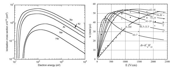
Figure 8.2: Left: Ionisation cross-section of the five lightest noble gases versus the energy of an incident electron. Heavier atoms have a larger cross section for a given electron energy [132]. Right: Electron drift velocity in argon-isobutane for different concentrations versus the external electric field. Even a small fraction of quenching gas modifies the shape of the graph significantly leading to higher drift velocities for smaller electric field [133].
