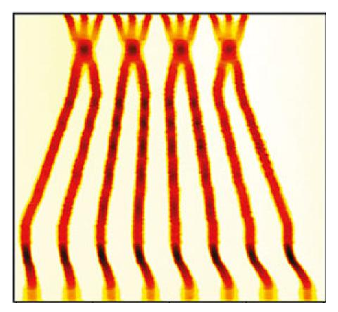
Figure 3.6: Beam splitting in the Proton Synchrotron using the Batch Compression Merging and Splitting (BCMS). The abscissa allows the identification of individual bunches while the time evolution is is shown on the ordinate axis [41].
