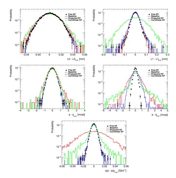
Figure 8.16: Smoothed resolution at the innermost surface of the tracking detector for 10 GeV initial momentum particles.
