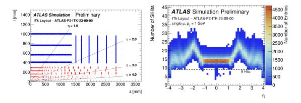
Figure 3.22: Left: Layout of the ITk. The location and radial distance of sensitive modules are shown versus z. Only the half z > 0 mm is shown. The red elements belong to the pixel detector, the blue elements to the strip detector. Right: Number of hits obtained from the ITk versus pseudorapidity  $\eta$ . Both plots are taken from Reference [84].
