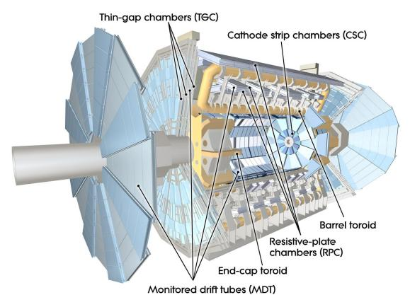
shown in Fig. 3.19. The components shown in this figure are described in the following,
