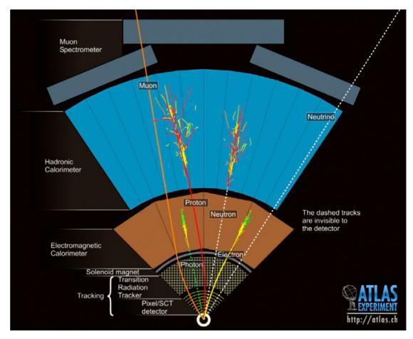
Figure 3.13: Cutaway overview of different particles traversing the barrel of the ATLAS detector in radial direction. The beam pipe is shown as white circle at the bottom [61].
