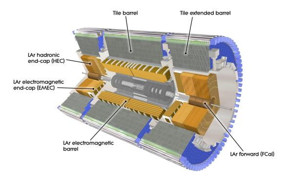
Figure 3.17: Cutaway overview over the ATLAS LAr and Tile Calorimeter [76].
