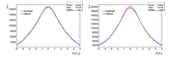
Figure 8.12: Pull distributions of predicted and filtered parameters obtained for the Projected KF at the point of filtering in the TPC with 1 GeV initial momentum. The statistics refer to the filtered distributions.
