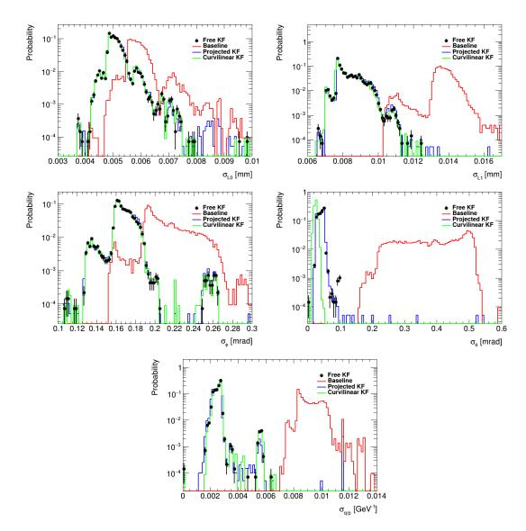
Figure 8.18: Smoothed uncertainty at the innermost surface of the tracking detector for 10 GeV initial momentum particles.
