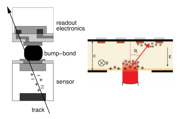
Figure 3.16: Left: Sketch of a hybrid pixel detector. A particle track ionises atoms in the sensor volume [66]. Right: Sketch of the deflection of electrons by the Lorentz angle  $\Theta_L$  in a semiconductor due to the magnetic field *B* [68].
