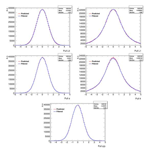
Figure 8.11: Pull distributions of predicted and filtered parameters obtained for the Projected KF at the point of filtering in the TPC with 10 GeV initial momentum. The statistics refer to the filtered distributions.
