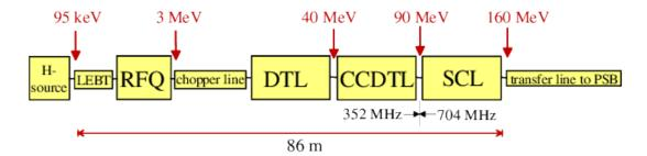
Figure 3.2: Schematic overview of the individual modules of the Linac4. Starting from the H<sup>-</sup> source on the the left, the individual acceleration steps are shown with the corresponding exit energies of the ion bunches [36].
