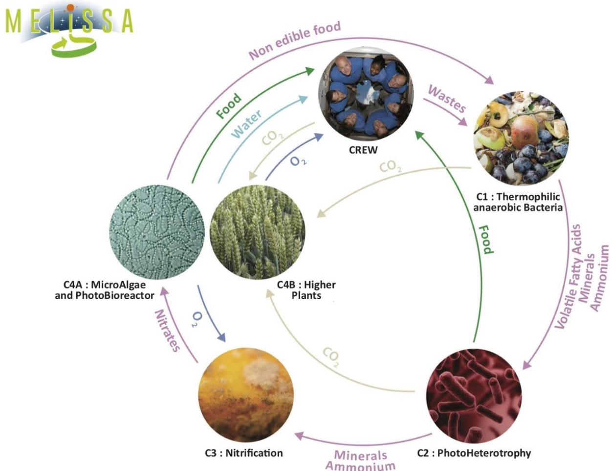
**Figure 2.3-1 A schematic representation of the MELiSSA loop, with the five compartments and their relations highlighted (Volponi and Lasseur 2020).**
