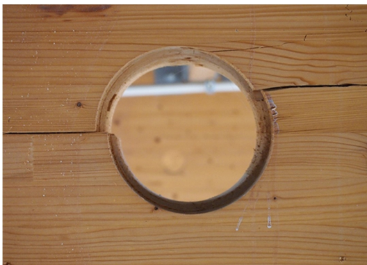
(c) Schubriss Durchbruch, u_{BSH} \approx 6\% (Dietsch 2017)
