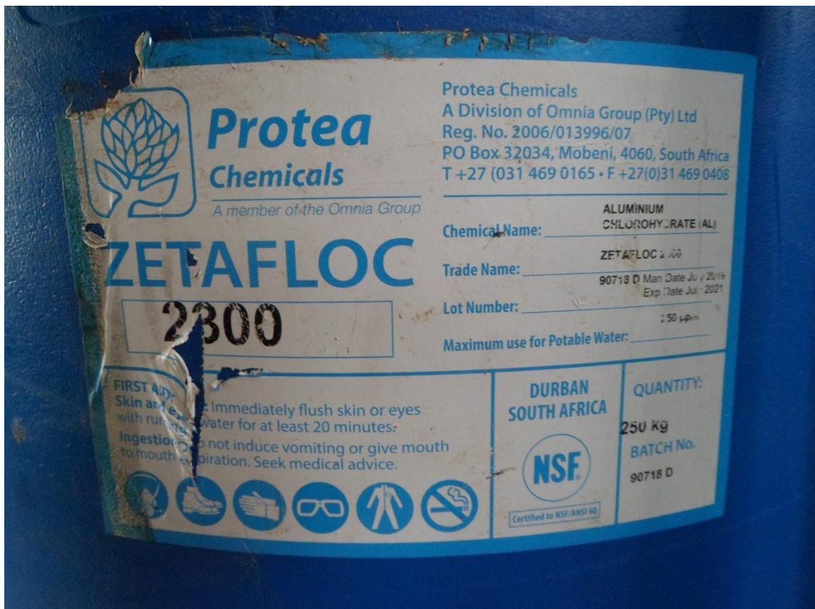
Ixix) The coagulant chemical (ACH) has the type designation "ZetaFloc 2300" and is imported from South Africa from the manufacturer Protea chemicals. The coagulant solution in the barrels is ready for application to the raw water stream and requires no further preparation.
