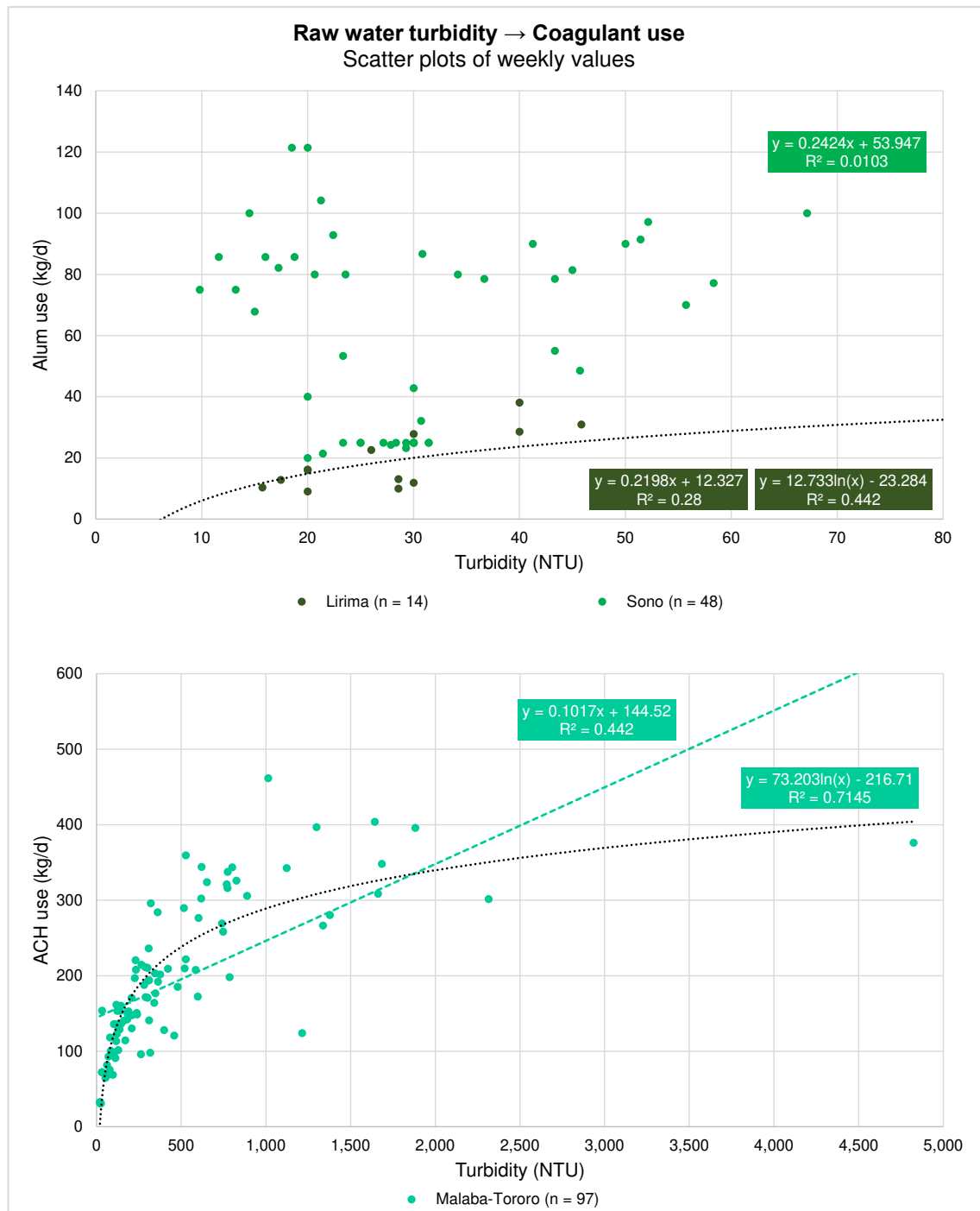
Figure 46: Scatterplot diagrams for the relationship of mean raw water turbidity to mean coagulant use at Lirima, Sono, and Malaba-Tororo DWTPs. Based on all available weekly values from September 2016 to January 2020. The linear regression graphs are provided with their functional equations and coefficients of determination ( R^2 ).
