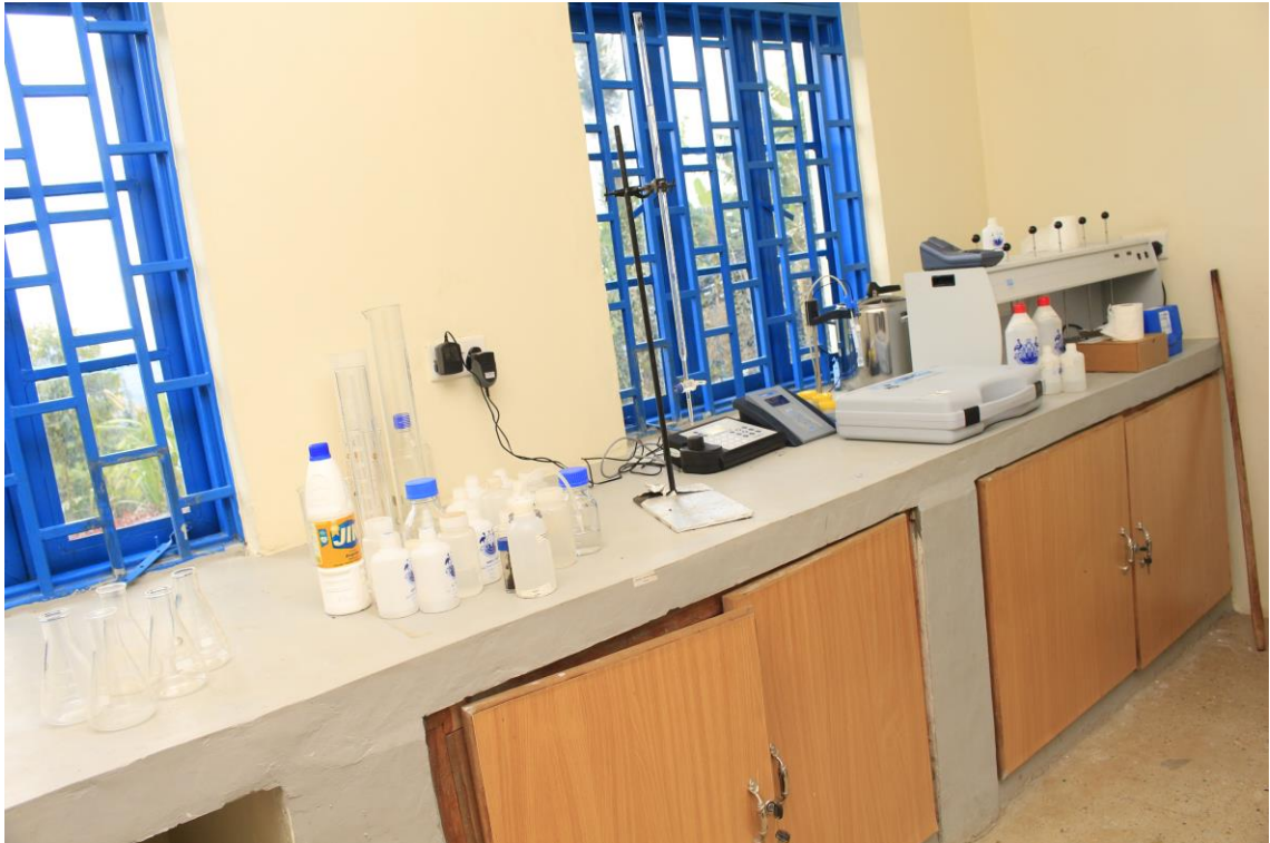
xxxvi) Laboratory at the DWTP of Lirima. Different water quality analyses for raw, clarified, filtered, and final water samples are performed, including for the parameters turbidity, hardness, alkalinity, pH, electrical conductivity, residual aluminium, and residual chlorine. Furthermore, jar tests to determine optimum coagulant doses, as well as chlorine demand tests to determine optimum disinfectant doses are carried out. According to John Ogire, the laboratory is equipped with the following devices: floc tester, photometer, microbiology kit, pH comparator, and turbidimeter tube. Photo by Elias Okemer.
