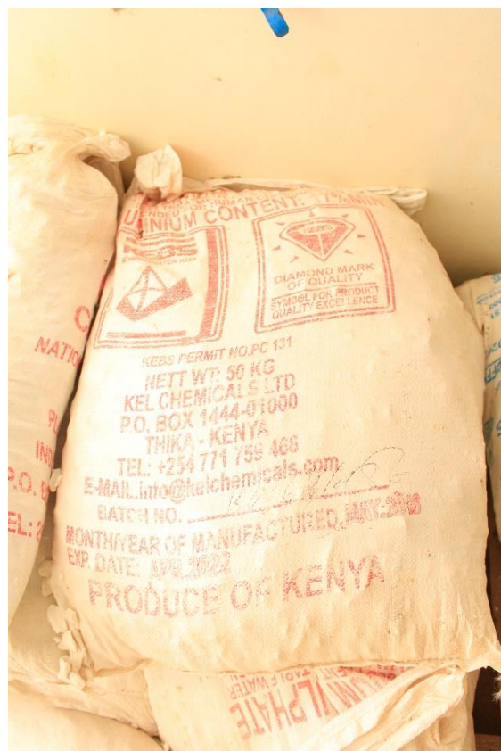
xxxix) Stored coagulant chemical (aluminium sulphate), imported from Kenya. Photos by Elias Okemer.
