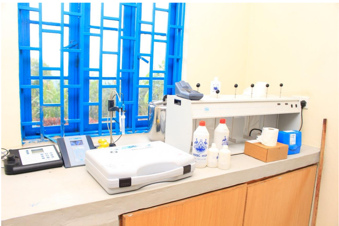
xxxvii) Laboratory equipment. From left to right: Lovibond T3 300 IR turbidimeter; Hach Sension+ MM 374 GLP 2 channel laboratory kit for pH, electrical conductivity, and others; jar testing device. Photo by Elias Okemer.
