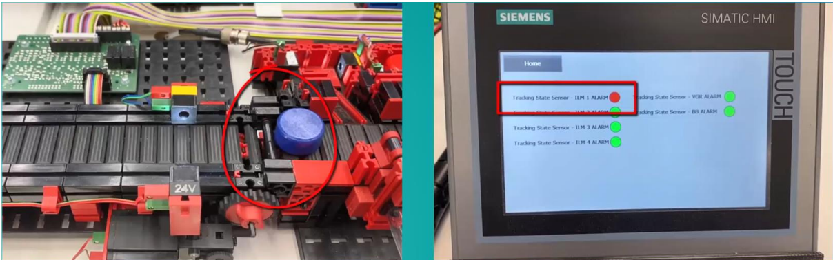
Figure 5.2: An alarm is triggered by Process Simulate due to a stuck product
