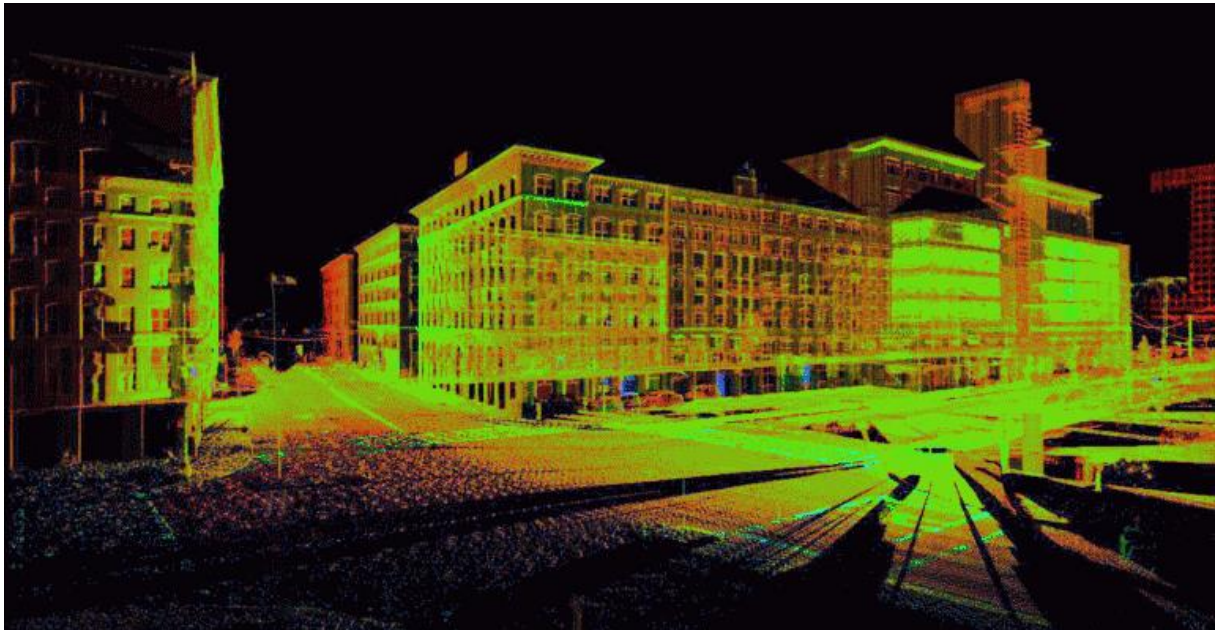
Figure 2.3: 3D laser scanning of sample infrastructure & buildings (LandTech, 2021)
