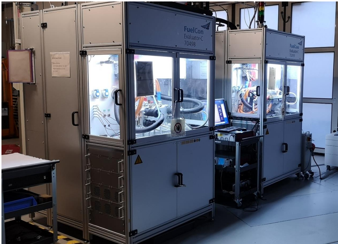
Figure 5: Two Horiba FuelCon test benches of the type Evaluator C1000-LT.
