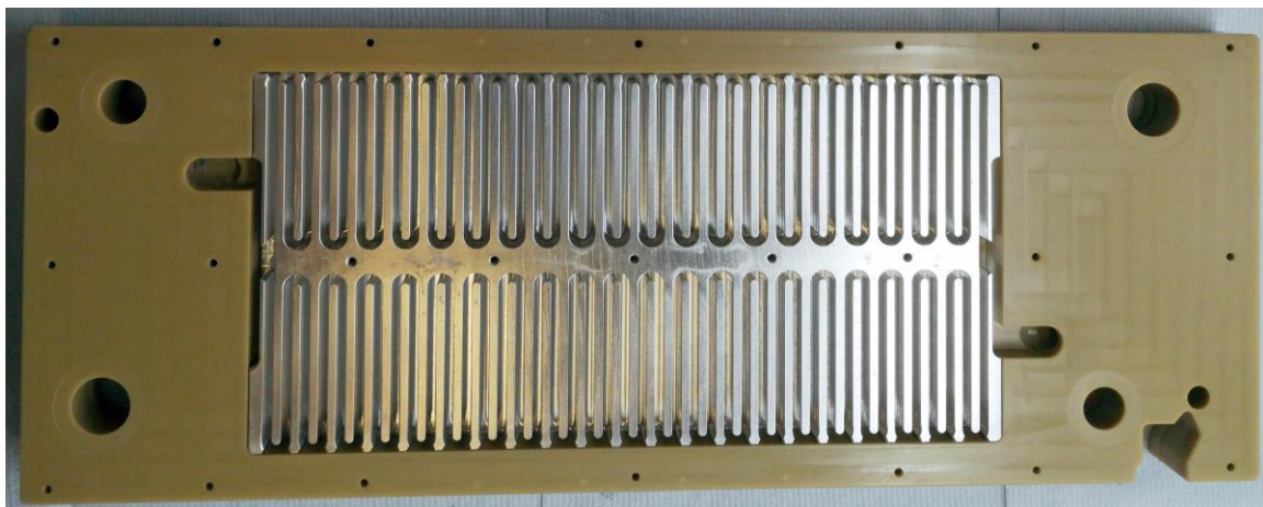
Figure 39: Underside of the aluminum heat transfer plate with the visible cooling channels in the assembled state with the water-conducting plate made of Ultem™.
