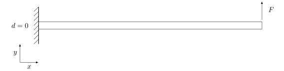
Figure 4.1.: Two dimensional simulation setup of the static beam bending scenario
