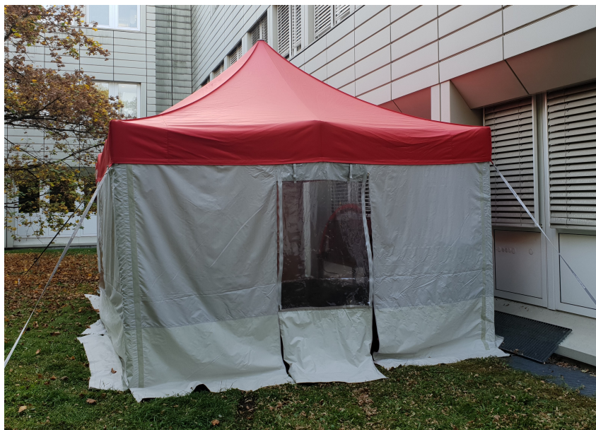
Figure 7.18: The soot generator could not be installed in the building and the biological labs. The solution we provided was this tent that we installed to protect the soot generator from the weather.
