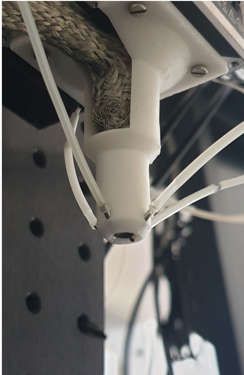
Figure 7.10: The scanning head of the four wavelength LD RSOM where the sample is illuminated from four side and the output of the fibers is not focused with a lens. All fibers and the UST are submerged into water.
