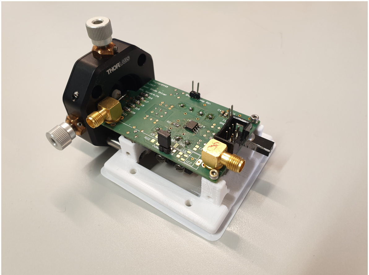
Figure 7.8: The final, updated, version of the pulsed laser diode driver that was used for all the experiments of Chapters 3-5.
