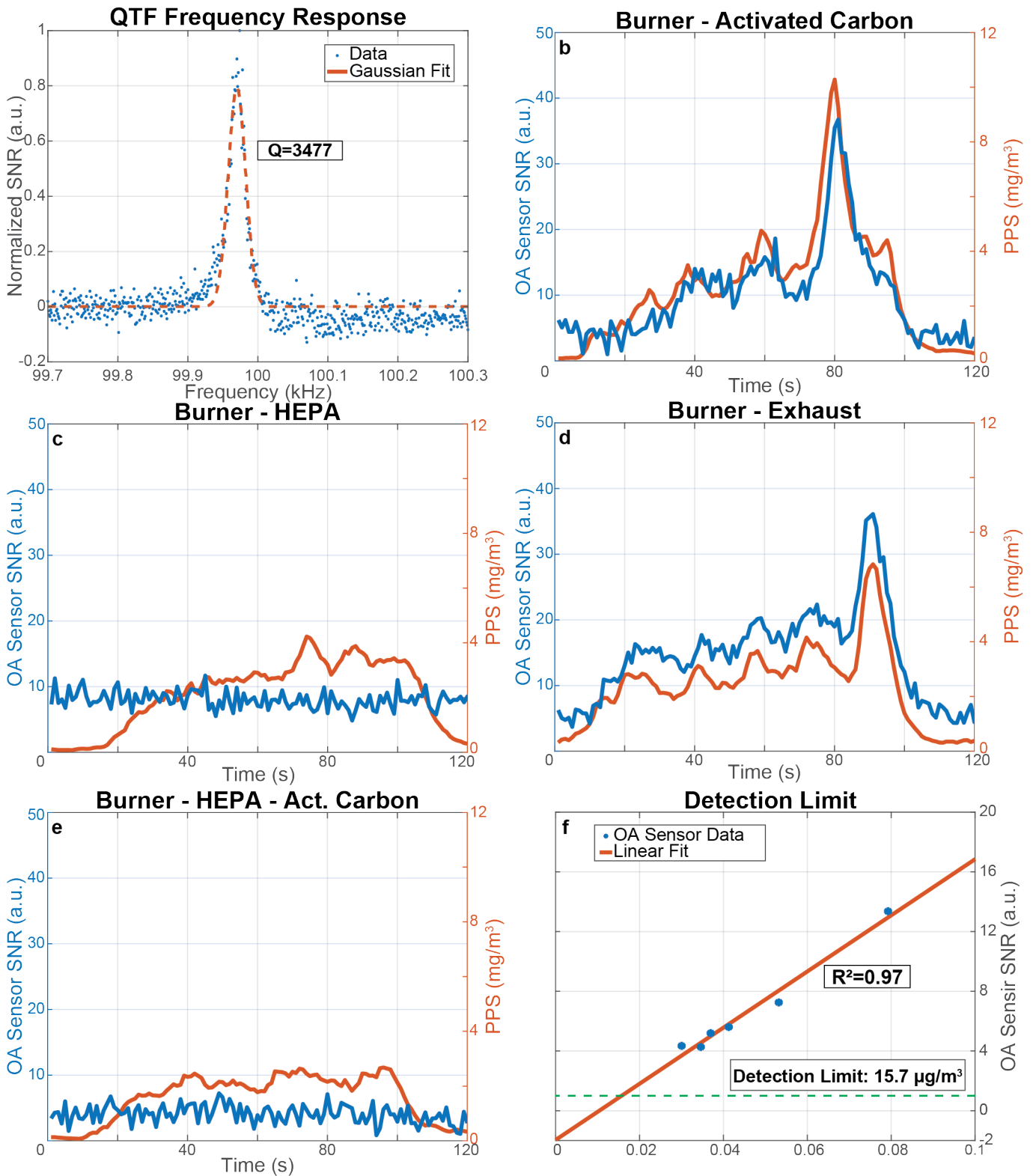
Figure 5.4: OA sensor characterization. (a) The frequency response of the QTF results in a Q factor of 3477. (b)-(e) OA sensor SNR as a function of time in high sooting mode with different exhaust gas treatment. (b) The exhaust gas after an activated carbon filter, (c) the exhaust gas after a HEPA filter, (d) the raw exhaust gas and (e) the exhaust gas after an activated carbon and a HEPA filter is detected. (f) the OA sensor SNR under different sample dilution ratios as a function of the PPS signal results in a detection limit of 15.7 \mu\text{g}/\text{m}^3 . Adapted version with permission from [289].
