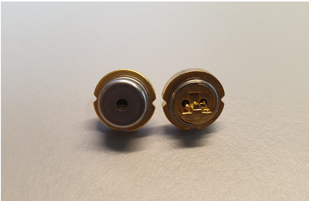
Figure 7.1: Two Continuous Wave Laser Diodes in TO-Can packages, one of which has its cap removed.
