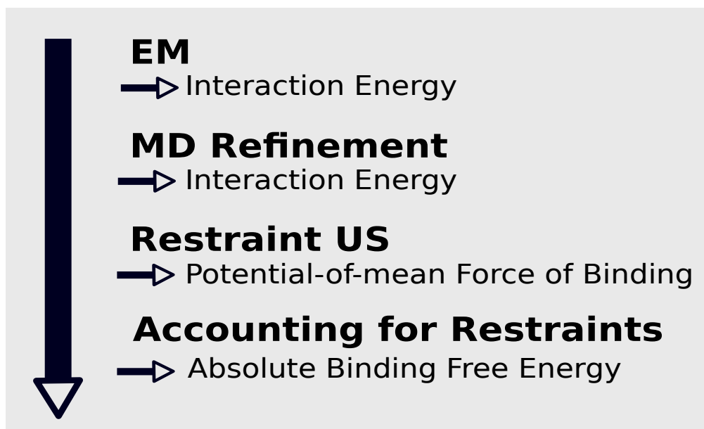
Figure 5.1: The different scoring methods that are used in this study. The binding energy was calculated after energy minimization (EM) and MD based refinement. Restraint umbrella sampling (US) yields the binding free energy and the absolute binding free energy was accessed by accounting for the restraints via the Woo and Roux scheme [324].
