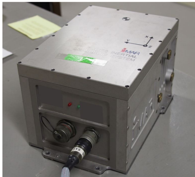
Figure 2.1: RQH housing with cable port on the backside. The b-frame axes are marked on top with the X axis pointing in front direction, the Y axis to the left, and the Z axis upwards.
