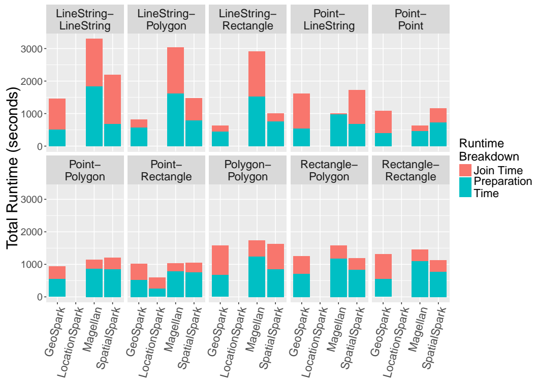
Figure 3.17: Total runtime cost breakdown for spatial joins between various geometric objects on a single node
