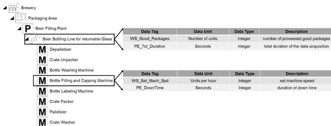
Figure 17. Plant model of the beer bottling line for returnable glass in use case 1
