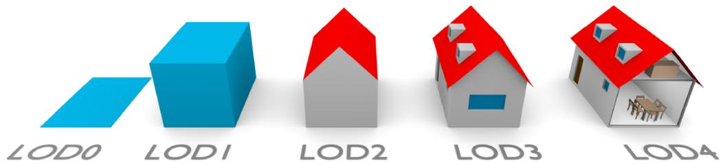
Figure 2.9.: Different Levels of Details in the CityGML standard [Biljecki, Stoter, Ledoux, et al., 2015]
