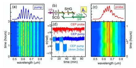
Fig. 4. Spectrum of the long time stable interference pattern from the f-2f interferometer obtained with the pump (a) and probe (c) pulses. (b) Setup of the continuum generation and second harmonic based f-2f interferometer. (d) Temporal evolution of the CEP of the pump (blue) and probe (red) pulses over 90 min. To demonstrate the CEP control we inserted, removed, and reinserted a 4 mm ZnSe plate after 10, 20, and 30 min (light blue).
