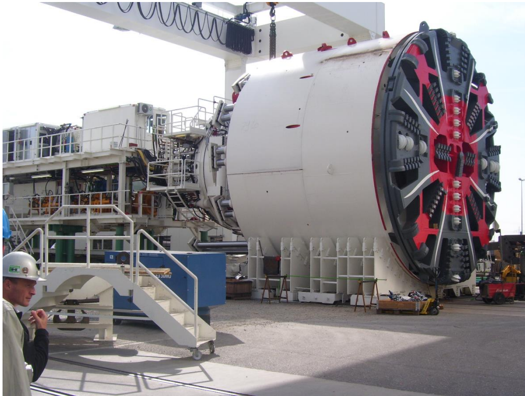
Figure 9-4 : Shielded TBM in suppliers' factory (source Herrenknecht)
