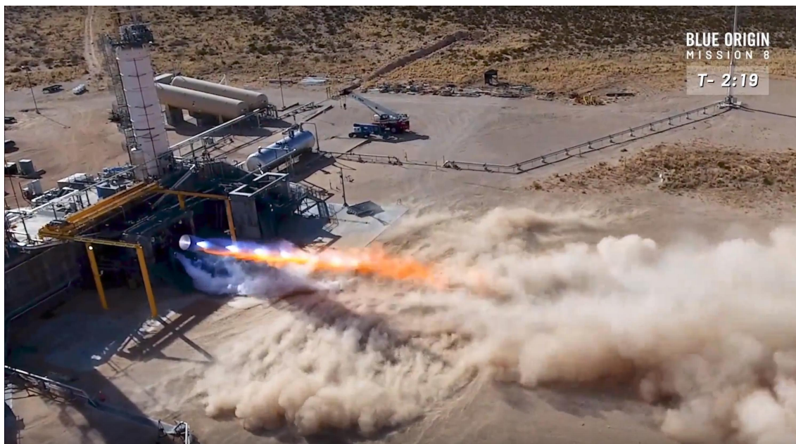
Figure 1.10: Full-scale hot-fire test of the BE-4 engine 8 .
