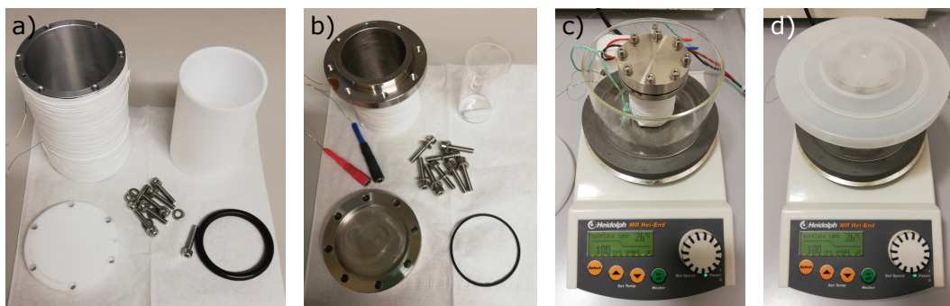
Figure 3.3: Disassembled stock solution thermostat (a) version 1 and (b) version 2. (c-d) Assembled version 2 stock solution thermostat on top of the magnetic stirrer. For additional thermal isolation a glass beaker with plastic hood is covering the device.
