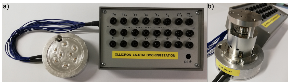
Figure 6.45: (a) Docking station consisting of the docking port and the patch field. (b) STM connected to the docking port.
