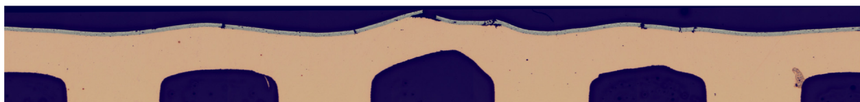
Fig. 17. Deformed shape of the central cooling channel structure of the coated specimen after 36 cycles, cross-sectional view.
