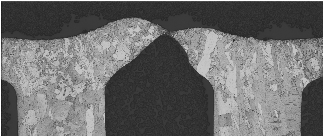
Fig. 10. 'Doghouse' failure in Campaign E (etched micro structure).
