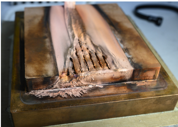
Fig. 13. Melted hot-gas wall in Campaign I.
