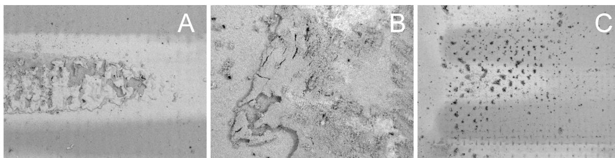
Figure 7.10: Optical microscope images of the anode substrate of C35 after 518 h of operation. A – Delaminated surface in the fuel channel. B – Accumulated material in the fuel manifold. C – Pattern of carbon particles where the nickel mesh had contact to the cell.
