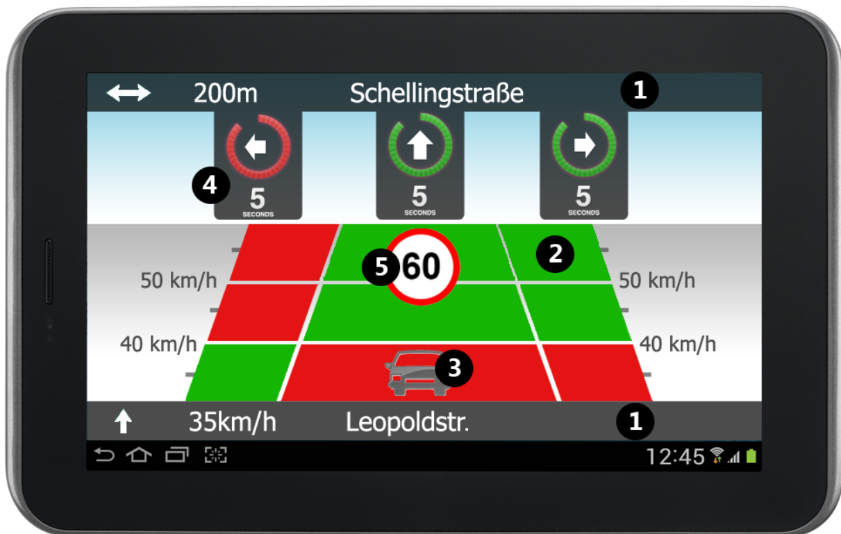
Figure 6.19: For running the online study, a base design with exchangeable elements has been created. Essential elements are ① information bars, ② speed carpets for indicating the speed range to cross the traffic light in the green phase, ③ current speed visualizations, ④ traffic light representations with remaining time, and ⑤ warning for violations of the speed limit.
