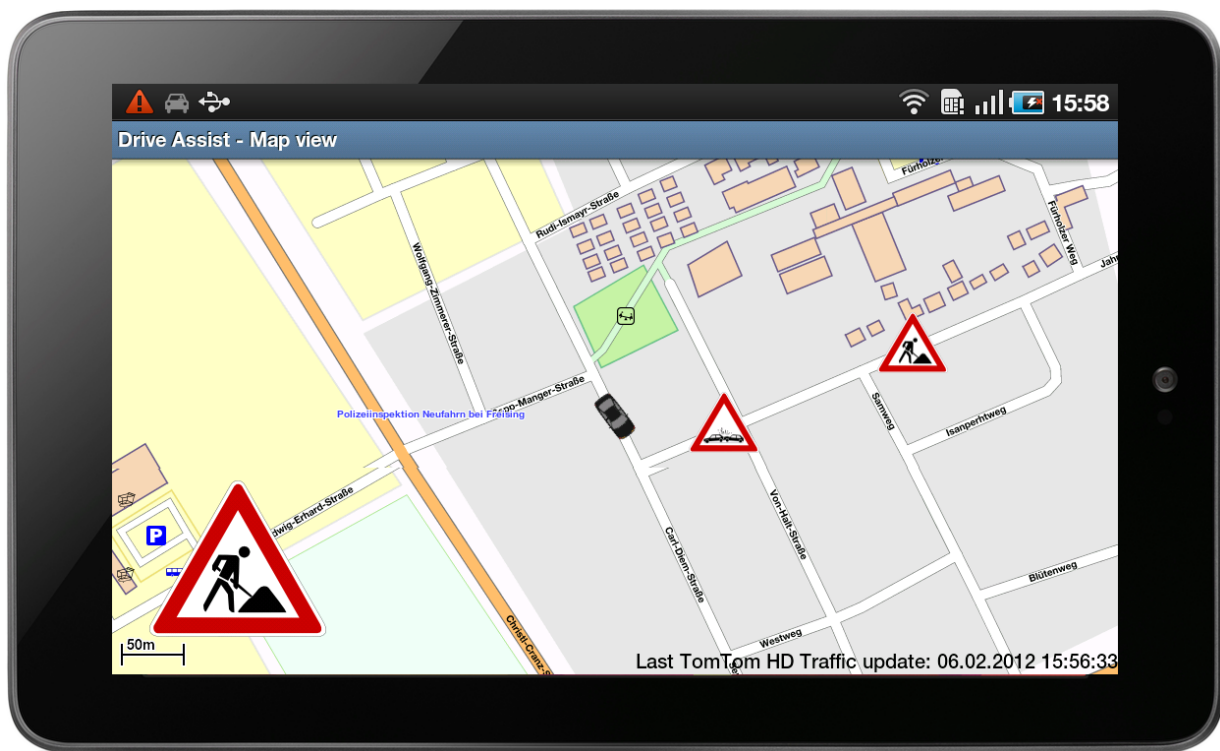
Figure 6.9: DriveAssist 's map view. The black car in the center represents the driver's vehicle. Newly received traffic events are indicated by the large traffic sign in the bottom left corner. The small traffic signs indicate the position as well as the type of the traffic event on the map.
