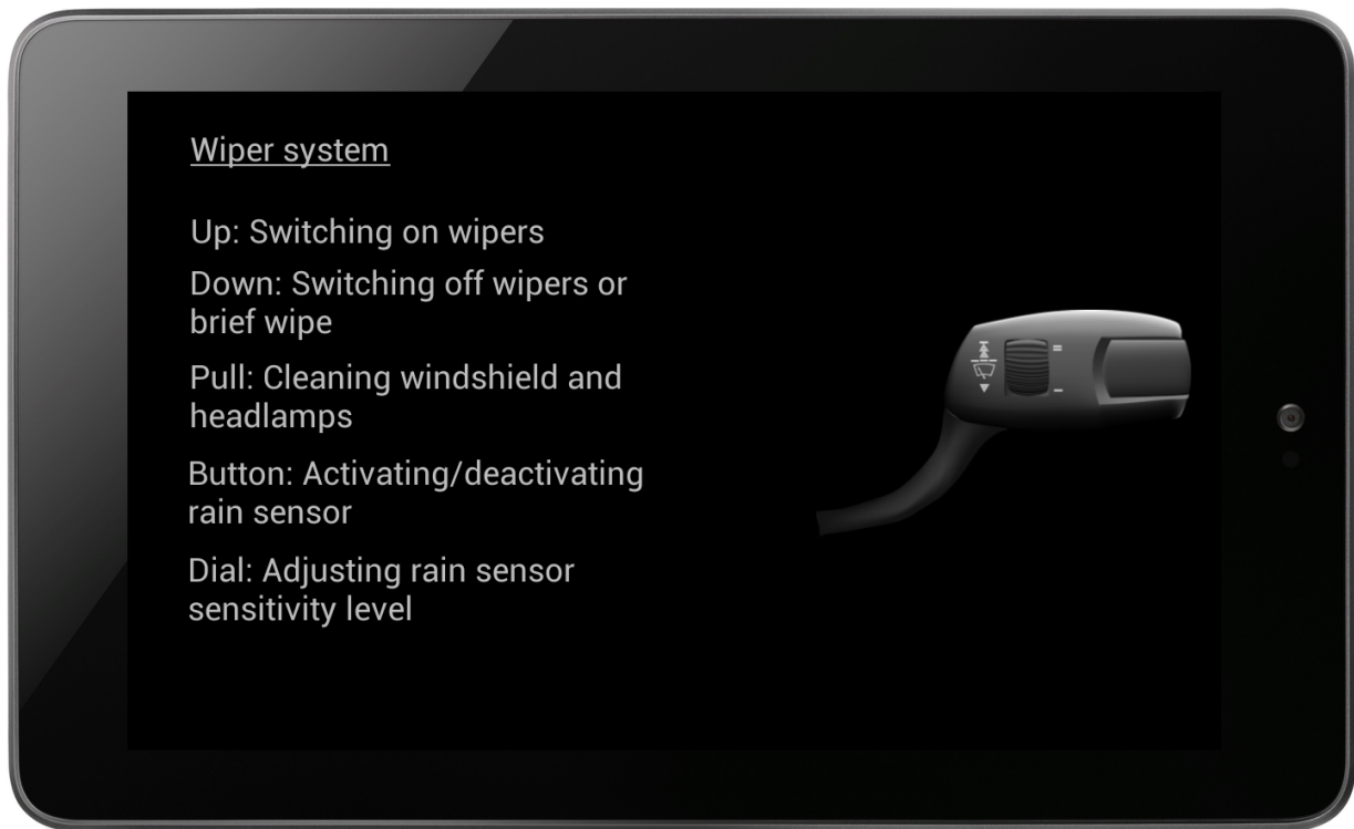
Figure 5.3: The details view explains the usage of the different interactive elements. There is also a walk-through for the vehicle’s infotainment menu. The example in this figure shows details on the wiper stalk switch.
