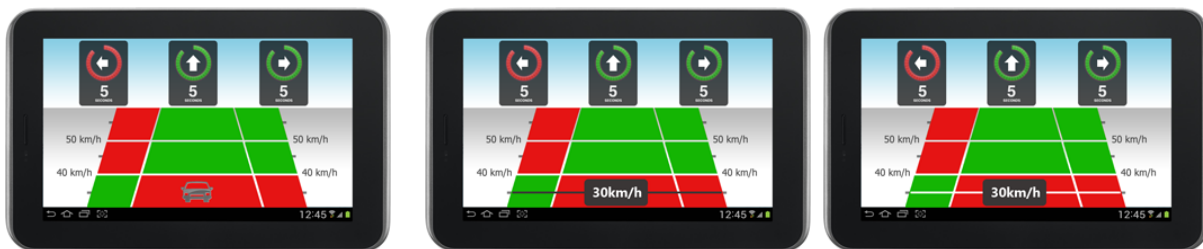
Figure 6.20: Design alternatives for the traffic light of the GLOSA prototype.
