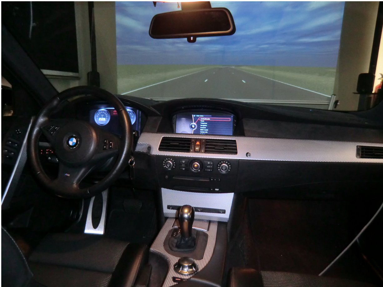
Figure 5.5: The user study on the effects of the gamified automotive user interface training took place in a driving simulator. It is the real cockpit of a BMW 5-series. The training application controls parts of the dashboard and the display on top of the center stack, and can log most controls by monitoring the vehicle's bus system.
