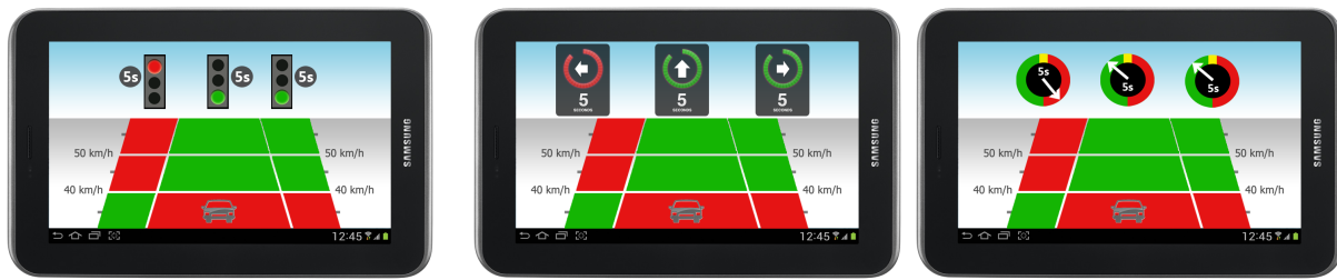
(a) Standard three-color traffic light. (b) Circular progress of remaining time. (c) Marshalite traffic signal with all phases at once.
