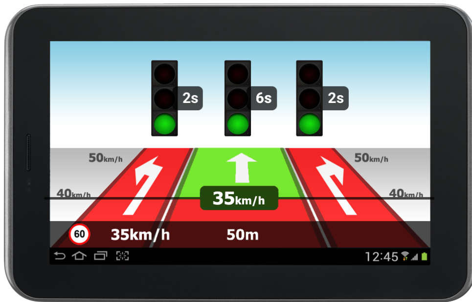
Figure 7.3: The experts initially rated the “color carpet” as not comprehensible. However, after a live demonstration in a simulated driving situation, they understood the approach. One expert summarized that the “[speed] carpet makes it easy since I only have to drive at a speed that [the black line] keeps in the green area.”
