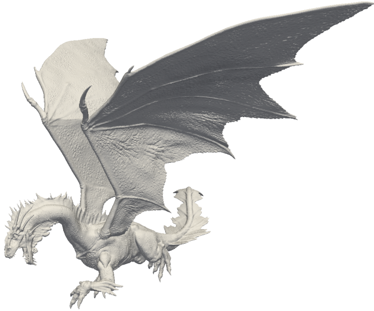
Figure 2.2: Boundary representation (STL format, 856 242 triangular elements) of a complex geometry, available free of charge at [138]. The inside of the model is hollow.
