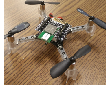
Fig. 5: CrazyFlie 2.0 quadrotor helicopter with UWB expansion.
