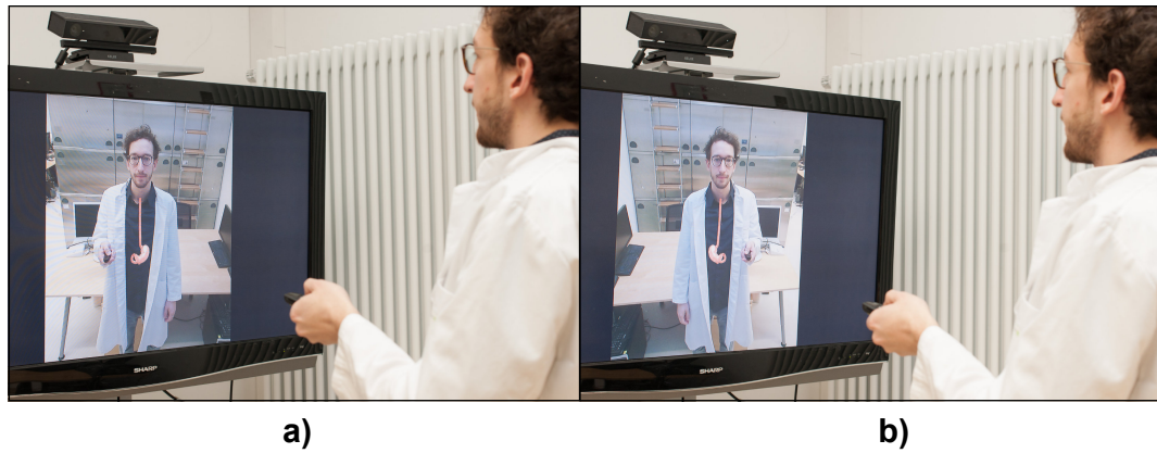
Fig. 3.10. "Spot the difference!" Comparison between a Reversing Magic Mirror (RMM) and a Non-Reversing Magic Mirror (NRMM). a) Similar to a real, physical mirror, left and right appear to be reversed in an RMM. Whereas the person in front of the system raises the left hand, the digital mirror image displayed on the TV screen raises the right hand; b) In the case of an NRMM, lateral inversion does not occur and the digital mirror image raises the left hand.
