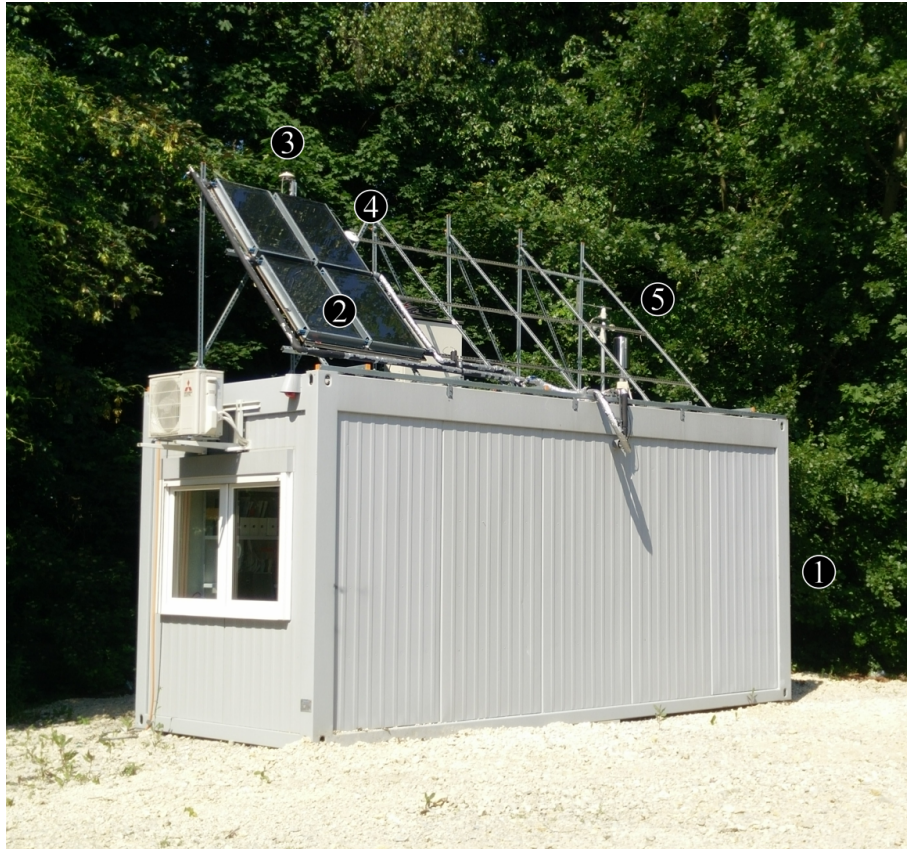
Figure A.2: External view of the system test rig. ① = Container, ② = Collector array, ③ = Pyranometer (horizontally mounted), ④ = Pyranometer (mounted under 45°), ⑤ = Weather station.
