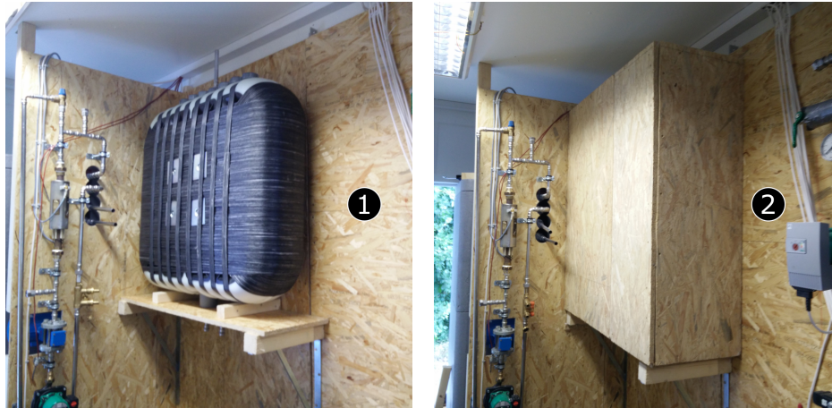
Figure A.5: Drain back reservoir of the system test rig. ① = Uncovered drain back reservoir, ② = Covered drain back reservoir. In order to minimise heat losses to the ambient, a pour-in insulation was filled in between the drain back reservoir and the wooden cover.
