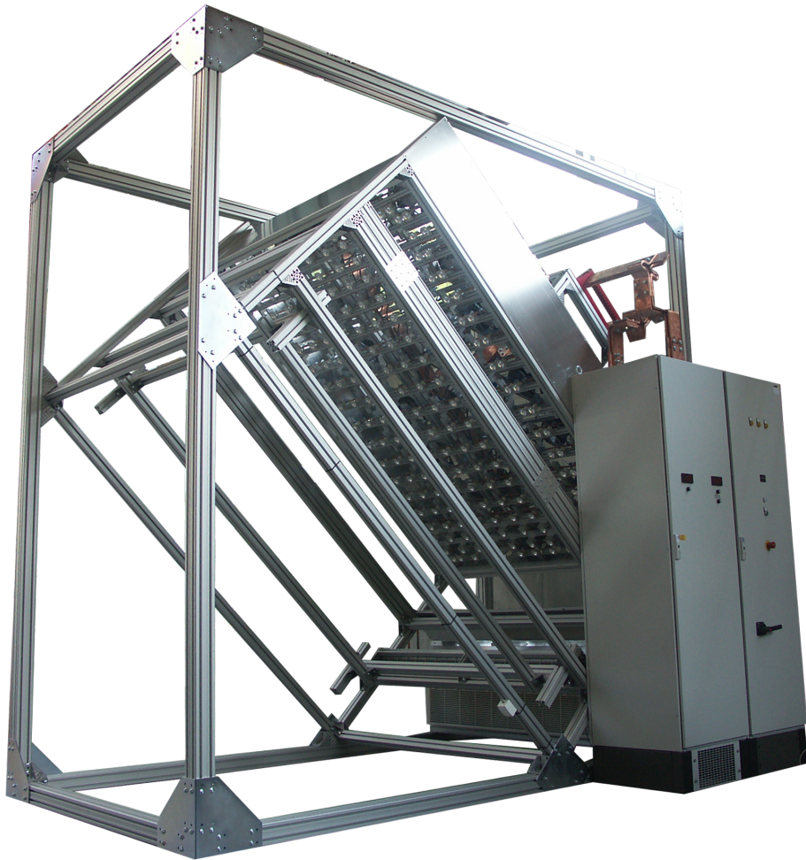
Figure A.7: Indoor solar simulator. 228 lamps provide a uniform level of irradiation ranging between 600 \text{ W/m}^2 and 1,100 \text{ W/m}^2 with a light spectrum comparable to the sunlight. A solar thermal FPC (maximum possible dimensions 1.4 \text{ m} (width) \times 2.3 \text{ m} (height), not shown in the photograph) is placed below the lamp field at an angle of inclination of 45^\circ . Fans above the lamp field provide an airflow to prevent the lamps from overheating. During operation, the test rig demands an electric power of approximately 30 \text{ kW} .
