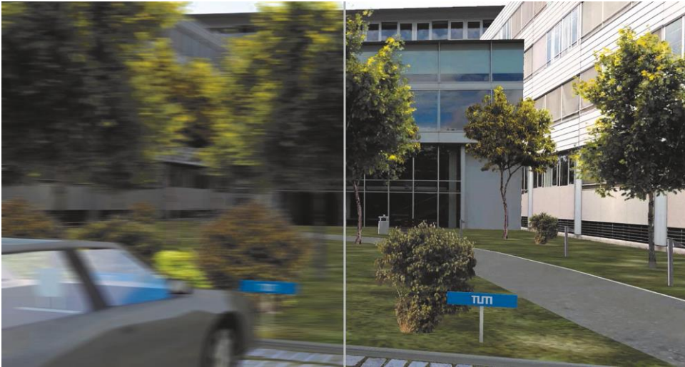
Figure A-2. Comparison of motion blur effects occurring in virtual scenarios with fast head movements: display configurations at full-persistence mode (left) and low-persistence mode (right).
