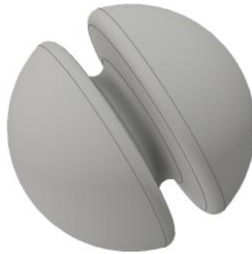
Figure 7.5: One of presumably a range of possible shapes capable to fulfill the requirements in regard to geometric surface area and pressure drop.
