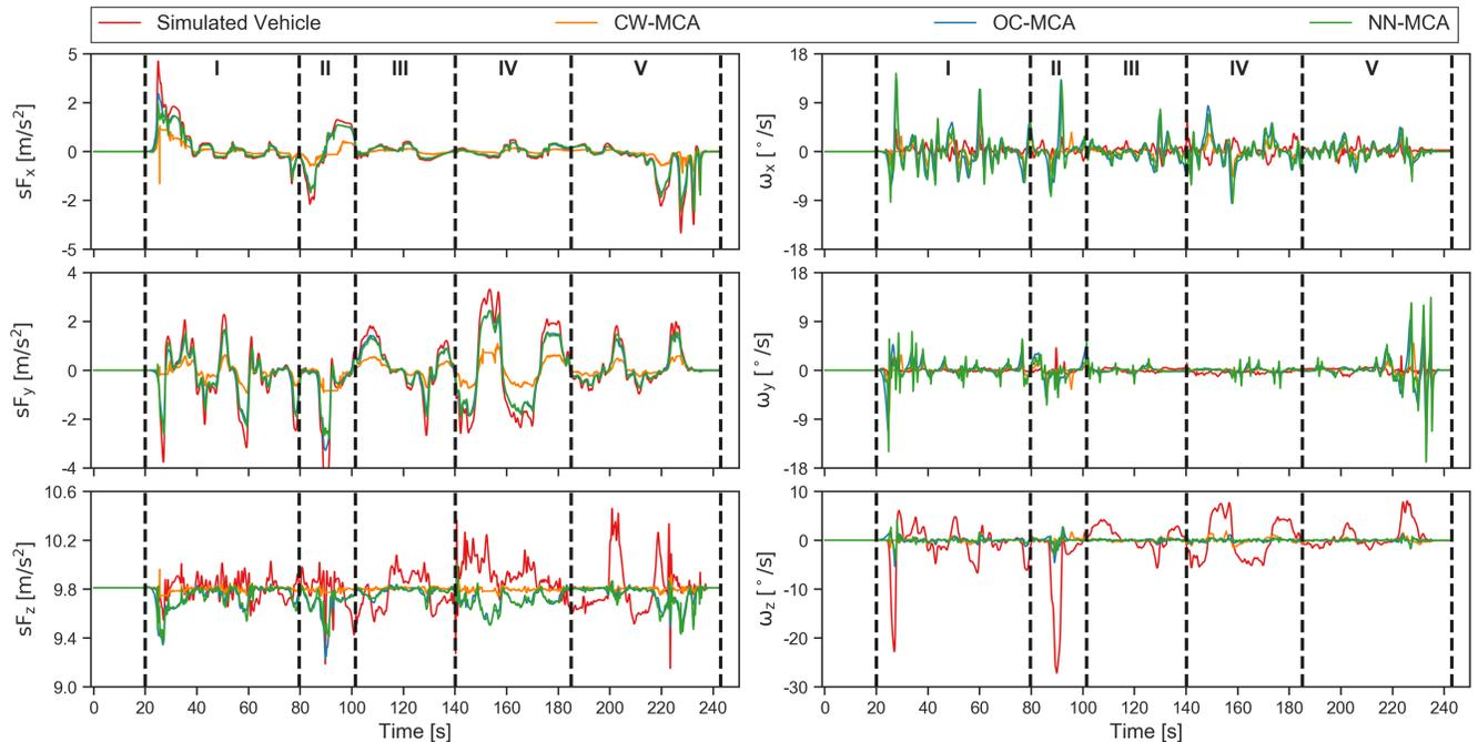
Fig. 6. The specific forces  $s\mathbf{F}$  and angular velocities  $\boldsymbol{\omega}$  of the simulated vehicle and the ones achieved by the Classical Washout (CW), Optimal Control (OC), and proposed Neural Network (NN) based MCA for an arbitrary trial from the test dataset
