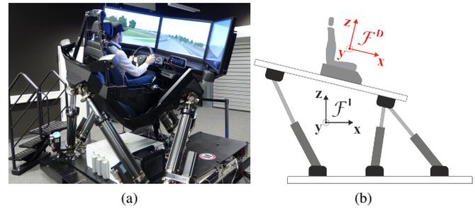
Fig. 1. (a) The dynamic simulator including the hexapod motion system manufactured by Cruden [9] used in our work. (b) Illustration of the used dynamic simulator with the inertial coordinate system  $\mathcal{F}^I$  of the simulator and the body-fixed coordinate system  $\mathcal{F}^D$  (driver’s coordinate frame) in the real world.
