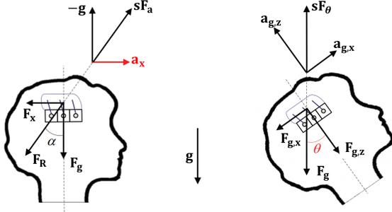
Fig. 2. The illustration of specific forces acting on human body under longitudinal acceleration (left) and rotation by angle  $\theta$  about y-axis (right) (adapted from [17]).
