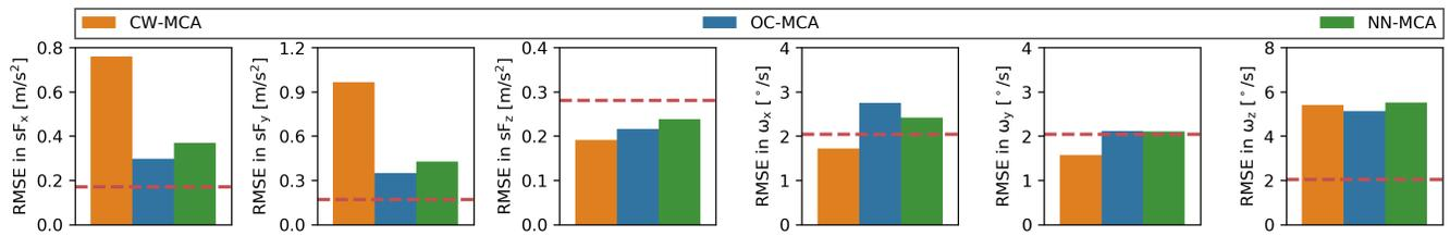
Fig. 5. The root mean squared error of the Classical Washout (CW), Optimal Control (OC), and proposed Neural Network (NN) based MCA in the test set for each DoF. The perception thresholds for each DoF are shown with red dashed lines.
