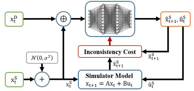
Fig. 4. Illustration of proposed NN-MCA during training. In the test phase, only the neural network part is used to generate (predicted) control commands ( $\hat{\mathbf{x}}_{t+1}^S, \hat{\mathbf{u}}_t^S$ ) for given driver's motion  $\mathbf{x}_t^D$  in the virtual world and simulator's current state  $\mathbf{x}_t^S$  in the real world. The operator  $\oplus$  corresponds to the vector concatenation of both inputs.
