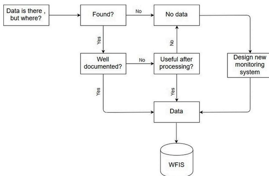
**Figure 6.** Schematic diagram for the followed processes to build the wellfield information system (WFIS).
