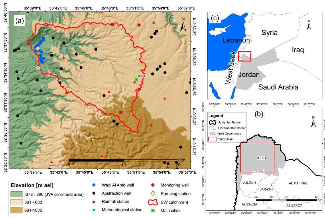
**Figure 1.** Overview map of the study area. (a) Shows the location the wells, rainfall stations, meteorological station, pumping stations and surface catchment area, it also shows the area topography. (b) Shows the area of Irbid governorate and the study area. (c) Shows the location of Jordan and surrounding countries.
