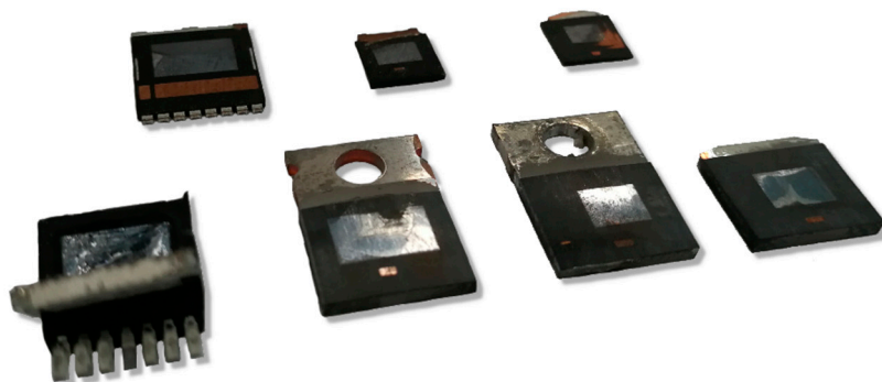
Figure 8. Opened switches from different manufacturers and with different electric parameters.
