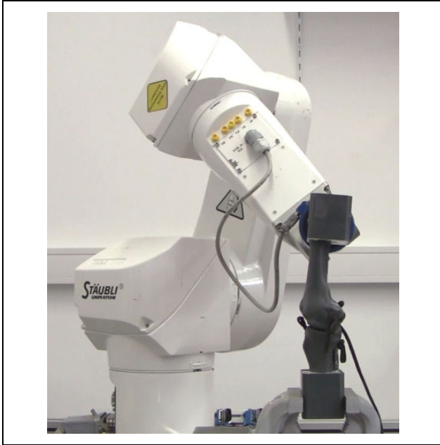
Figure 5. Test setup for the multi-force control. The robot is attached to an additive manufactured replica of the human knee joint.
