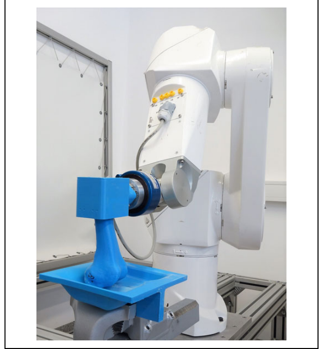
Figure 1. Experimental setup to evaluate the contact control. An additive manufactured femur replica is moved along a rigid oversized tibia plateau, which is cornered by rising edges.
