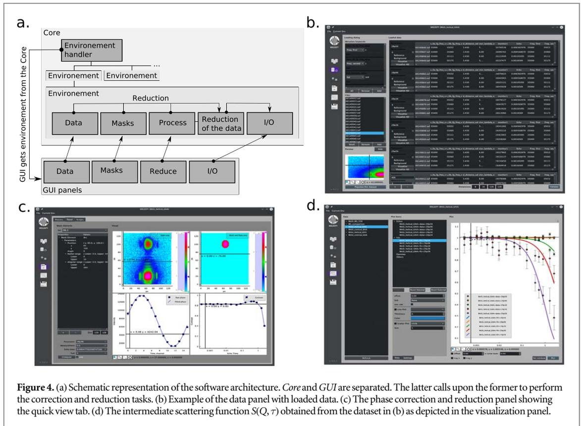
data reduction is organized in scripts which are filled and started by the GUI. Furthermore, the scripts can be edited directly to retain flexibility. The panel contains a quick view of the data that allows preliminary insights on what the reduction process might yield. This can be seen in figure 4(c).
