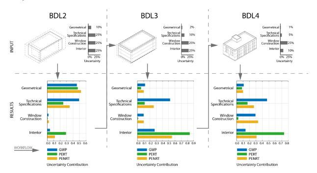
**Figure 2.** Input uncertainty (vagueness) in parameter groups and resulting uncertainty contribution for a rectangular building shape and reinforced concrete structure; exact numbers are listed in Appendix A, Table A1.
