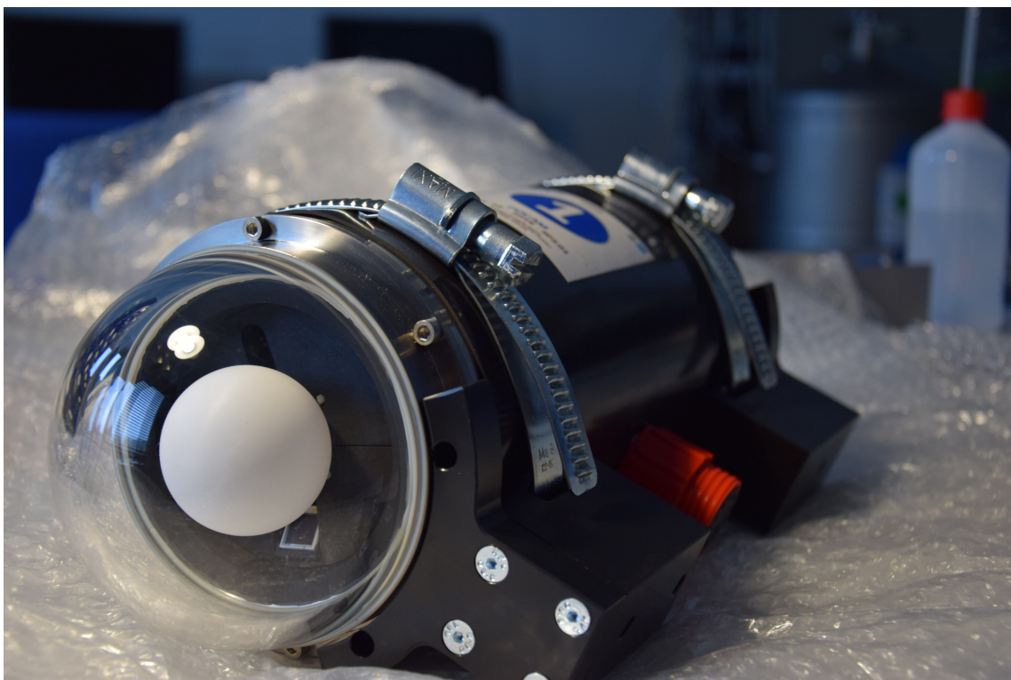
Figure 11. Finished POCAM module prior to shipment to Canada. Visible is the housing, one integrating sphere, the mounting structures and the instrument connector including its safety clamp.
