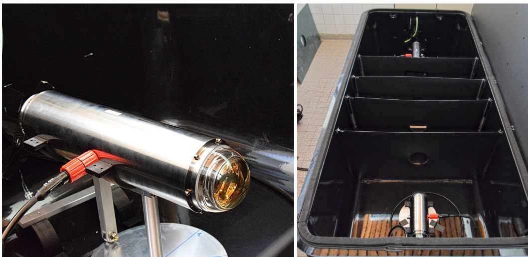
Figure 23. Wet test setup at TUM. The sDOM is fixed to a rotation mount inside a 3\text{ m} \times 1.2\text{ m} pool with baffles for suppressing reflected light. The pool is filled with water during the tests and closed by a light-tight lid.
