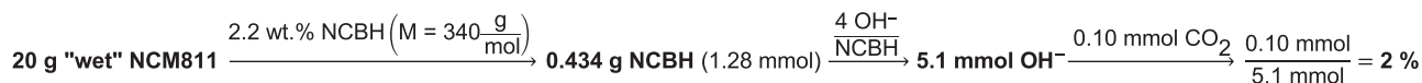
Figure 11. Overview of the model calculations of CO 2 generation due to the reactions of surface contaminants with the electrolyte component EC for a 3 Ah battery cell containing “wet” NCM811 as cathode active material.
