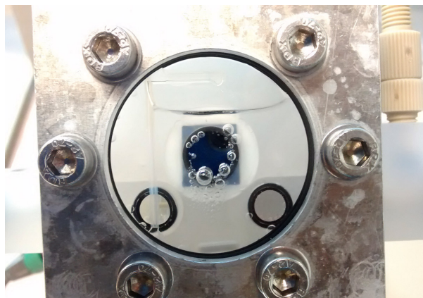
Figure 7.20: Picture of the EC-cell. The sample is mounted in the center of the EC-cell and sealed with an O-ring. It can be illuminated either from the backside or from the front through the electrolyte.
