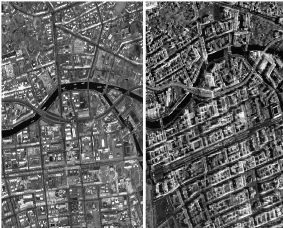
Fig. 8. Display of SAR-optical sub-scenes extracted from Berlin study areas (the left-hand image is from WorldView-2, right-hand image is from TerraSAR-X).
