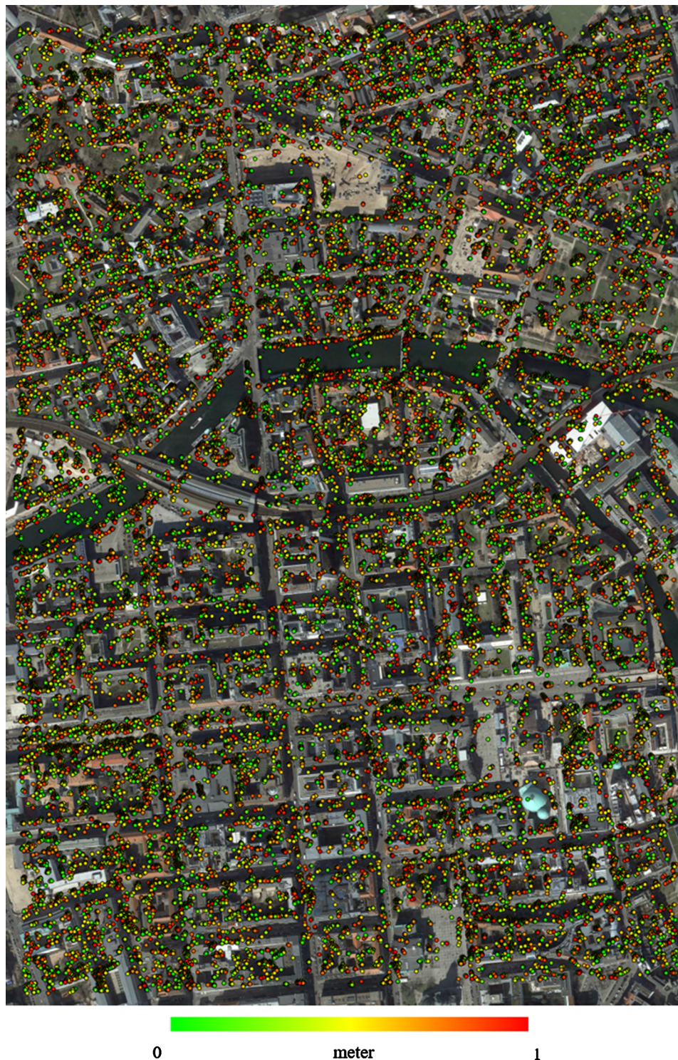
Fig. 21. Position of points with subpixel accuracy (1 m) achieved by dense matching over Berlin city.
